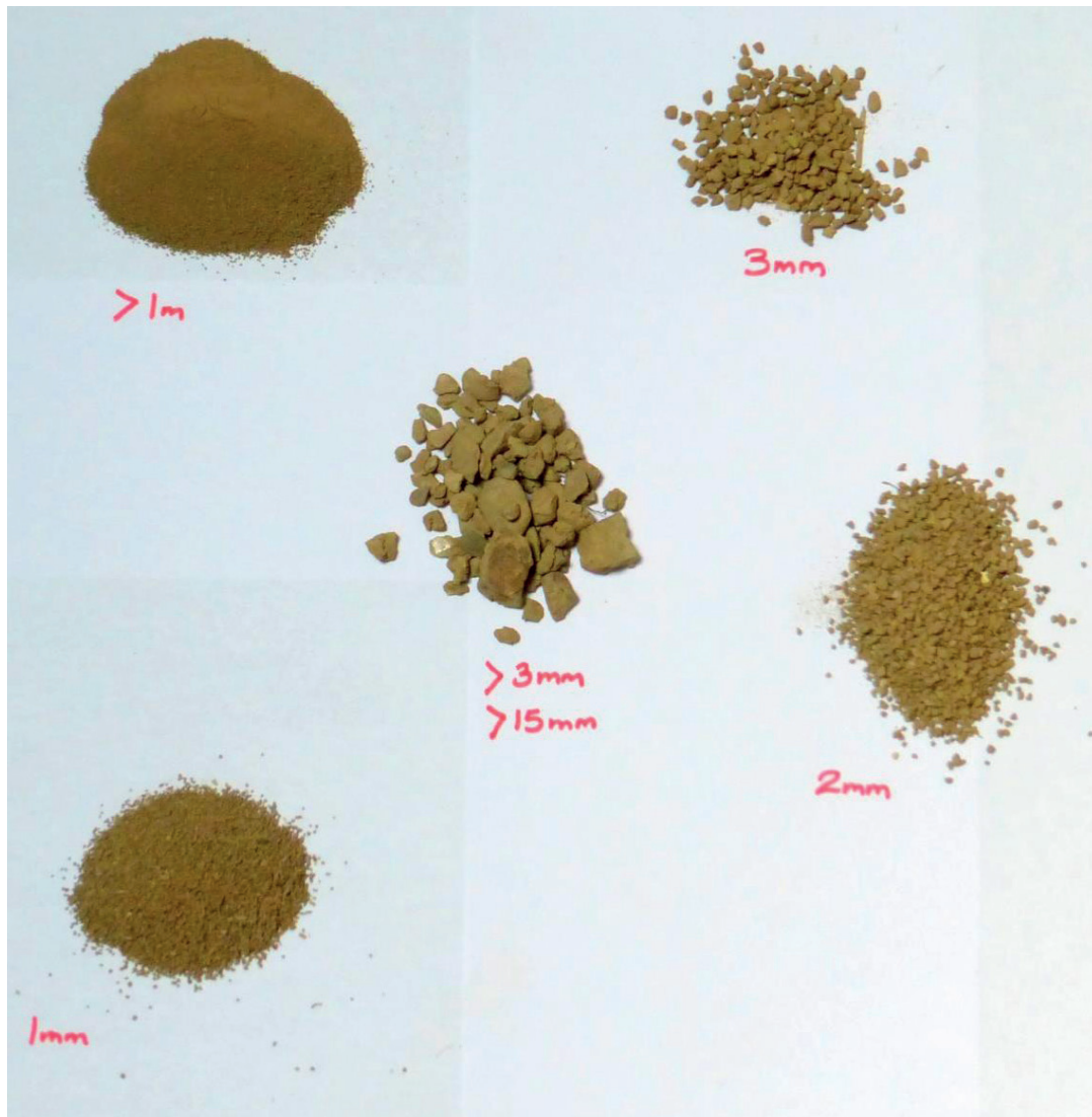
Fig.58. Analysis by John Alexander of the components of the earthen matrix at Merton. More detailed analysis from this and other sites is needed to better understand the composition of the earthen matrix for bedding and jointing above formation level and how this contributes to performance. John Alexander.
