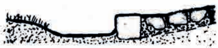
Squared kerbing dropping down to an intended, "earthen" gutter/ drain channel (e.g. Tiverton)
