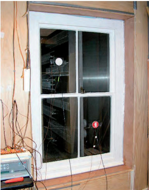
Left: Heat flux sensor positions on glazing; above sensor dimensions
