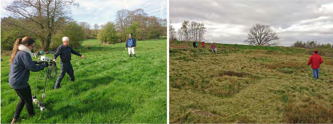
*Fig 13: Volunteers using a resistivity meter at Sheepwash Farm (left) and carrying out magnetometry survey over the medieval building platform within Castle Ring hillfort (right), April 2017 © Historic England.*
