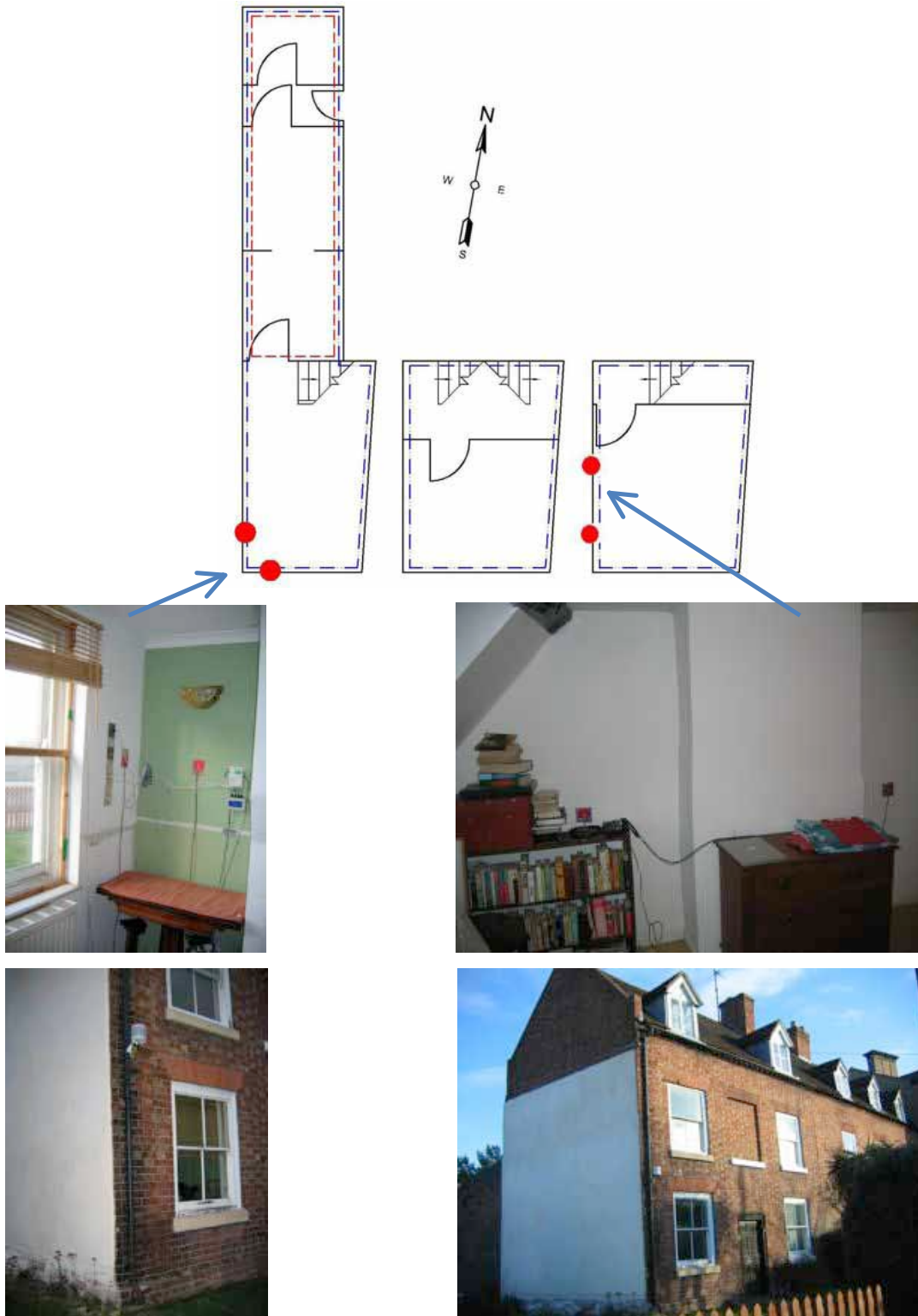
Figures 3 - 6. Showing positions of in situ monitoring equipment at 116 Abbeyforegate, Shrewsbury, 2011.
