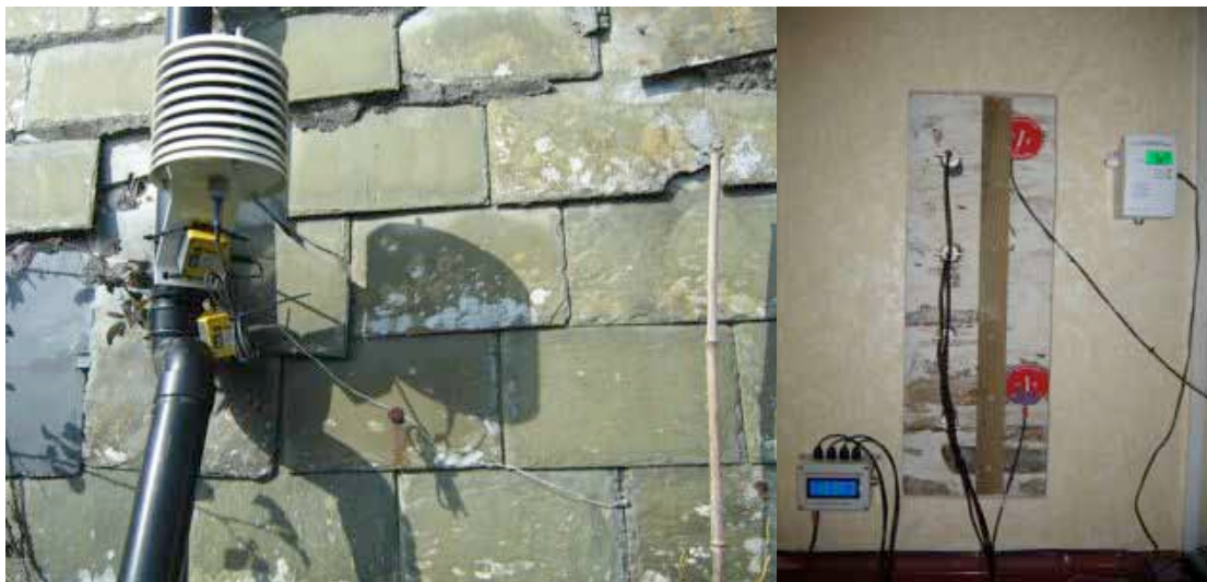
Figure 73. Positions of in situ monitoring equipment at Rock View, Devon Consols 2011.
