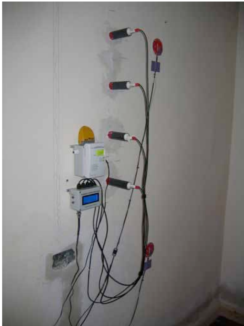
Figure 68. Interstitial, U-value and IAQ monitoring set up at Mill House, Drewsteignton, 2011.
