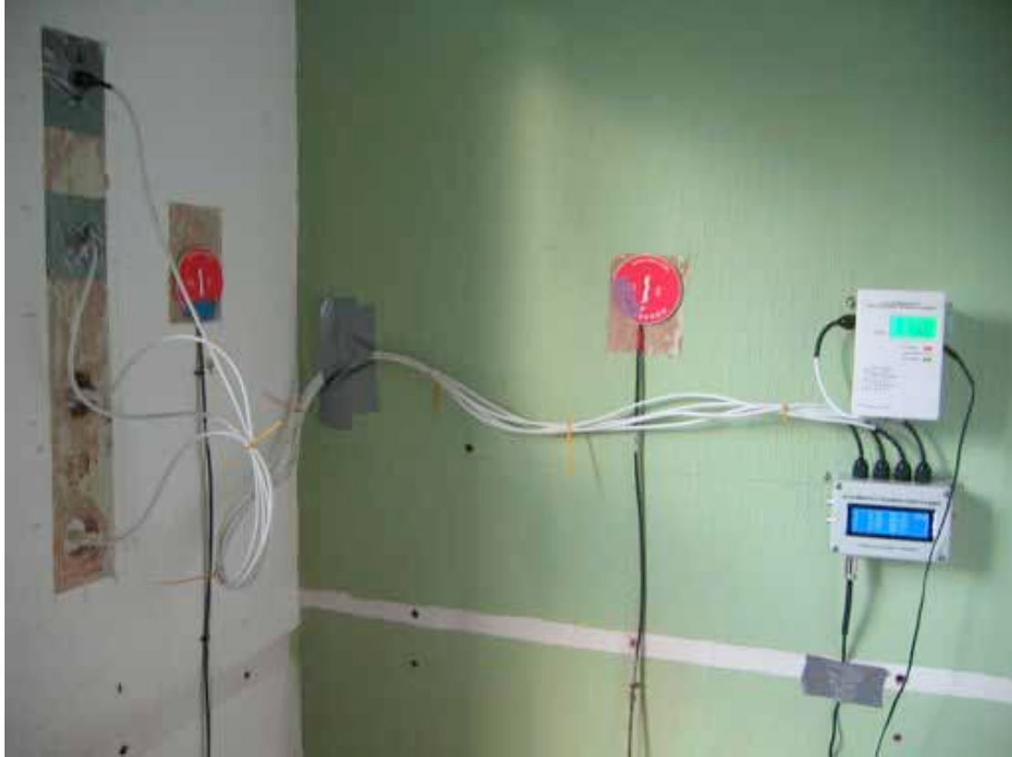
Figure 11. Interstitial, U-value and IAQ monitoring set up at Abbeyforegate, Shrewsbury, 2011.
