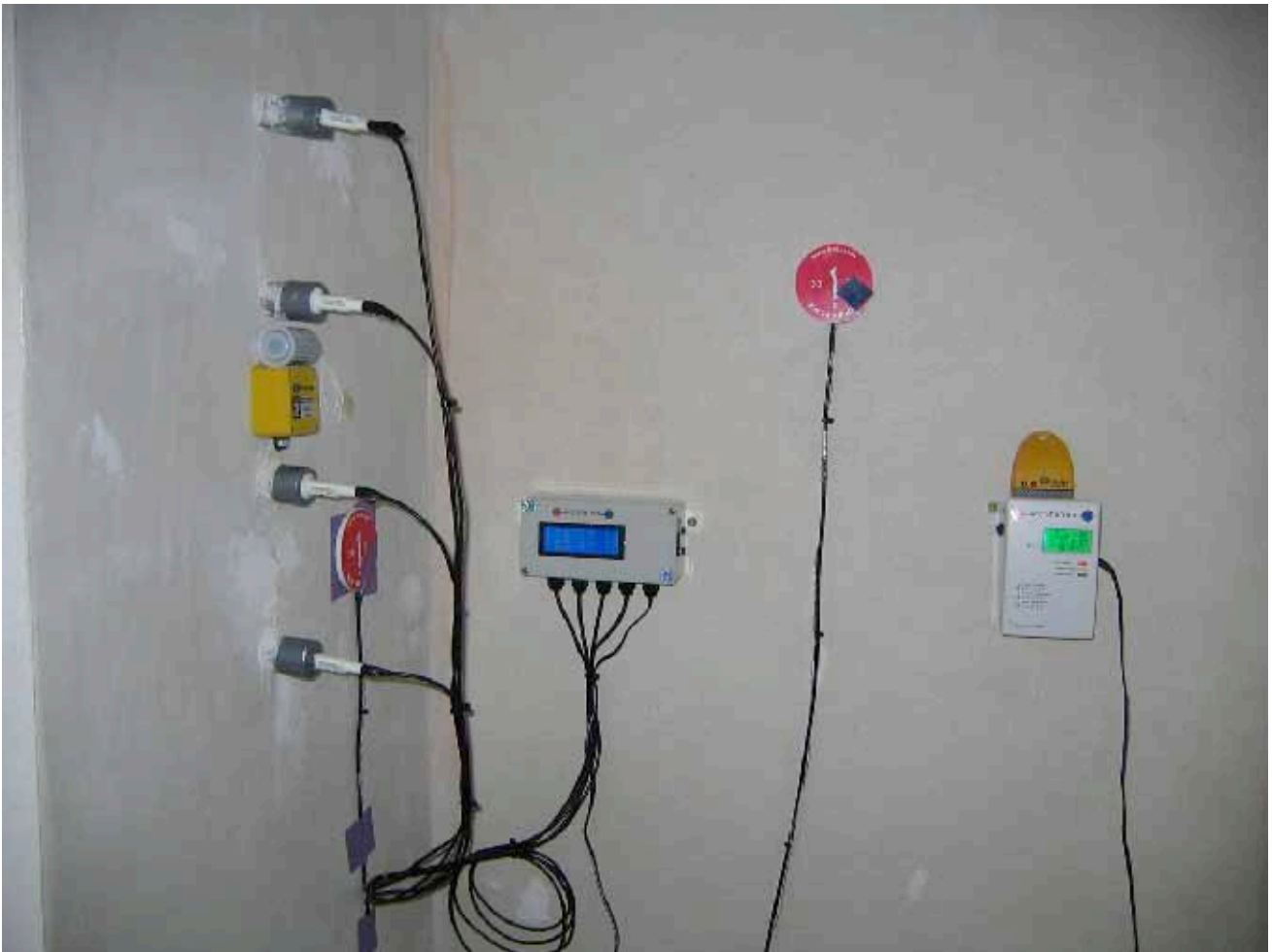
Figure 37. Interstitial, U-value and IAQ monitoring set up at Abbeyforegate, Shrewsbury, 2012.
