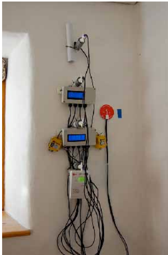
Figure 77. Interstitial, U-value and IAQ monitoring set up at The Firs, Riddlecombe, 2012.
