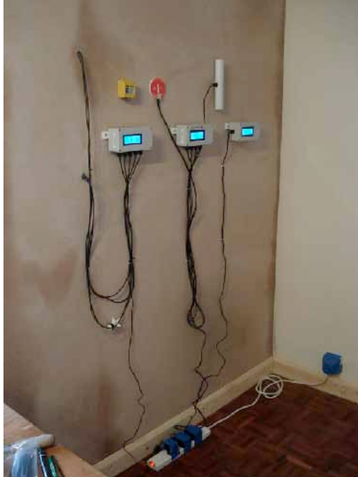
Figure 70. Interstitial, U-value and IAQ monitoring set up at Mill House, Drewsteignton, 2012.
