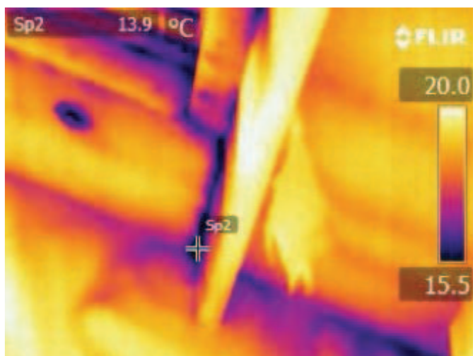
Figure 51. White House Farm, Stirton, Skipton □ ingress around roof light casement, beam, wall joint and light fitting in Utility Room.
