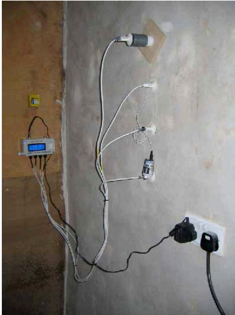
Figure 57. Interstitial monitoring set up at White House Farm, Skipton, 2013.
