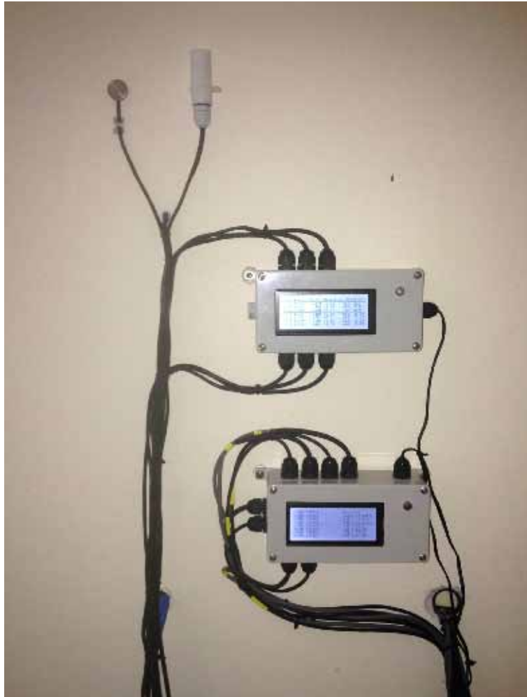
Figure 16. Interstitial Hygrothermal Gradient and Material Moisture Monitoring, Drewsteignton.
