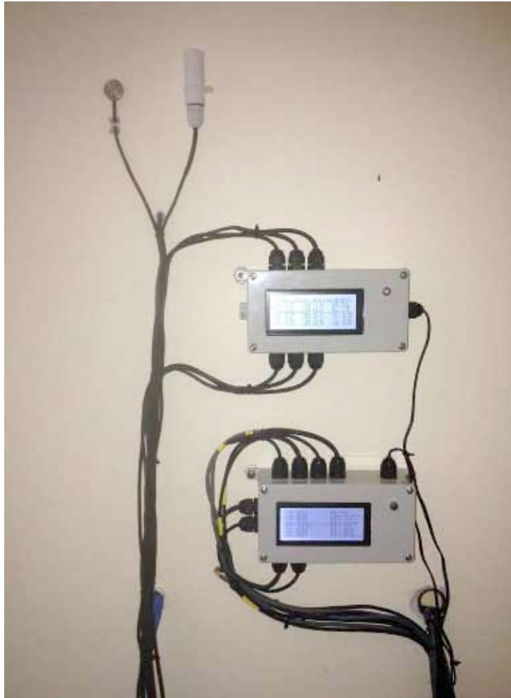
Figure 21. Interstitial hygrothermal gradient and material moisture monitoring, Drewsteignton.
