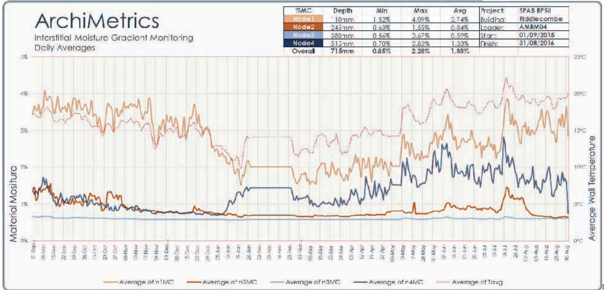
Figure 47. Material moisture content over time, The Firs, Riddlecombe 2015-2016.
