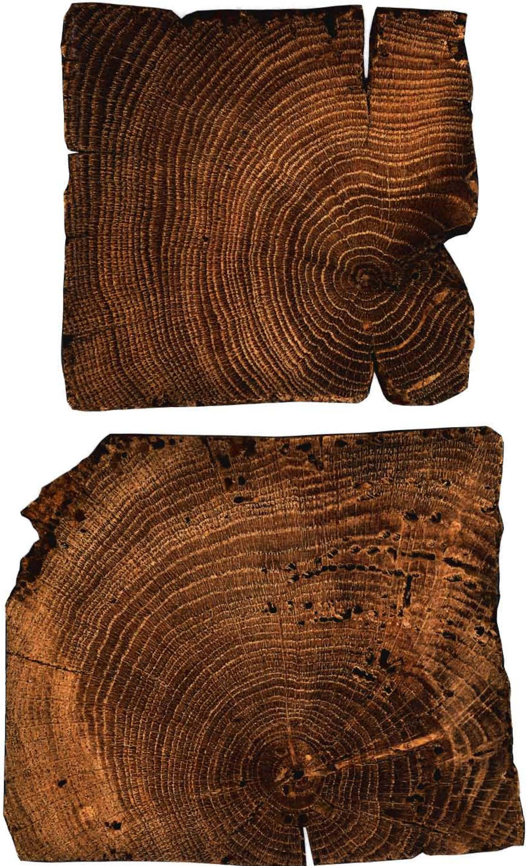
Figure 25: Typical examples of faster-grown English timbers - scec68 (south rafter T21, south chapel) and scec72 (south solepiece T10, north chapel) (90%)
