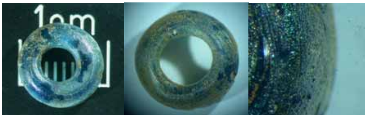
Figure 4. The stages of surface deterioration in the glass beads. Left: surface iridescence that is becoming detached (No. 200435027) Middle: the detaching surface has become brown due to decay Right: the surface has become scaly, and powdery as a result of further decay.
