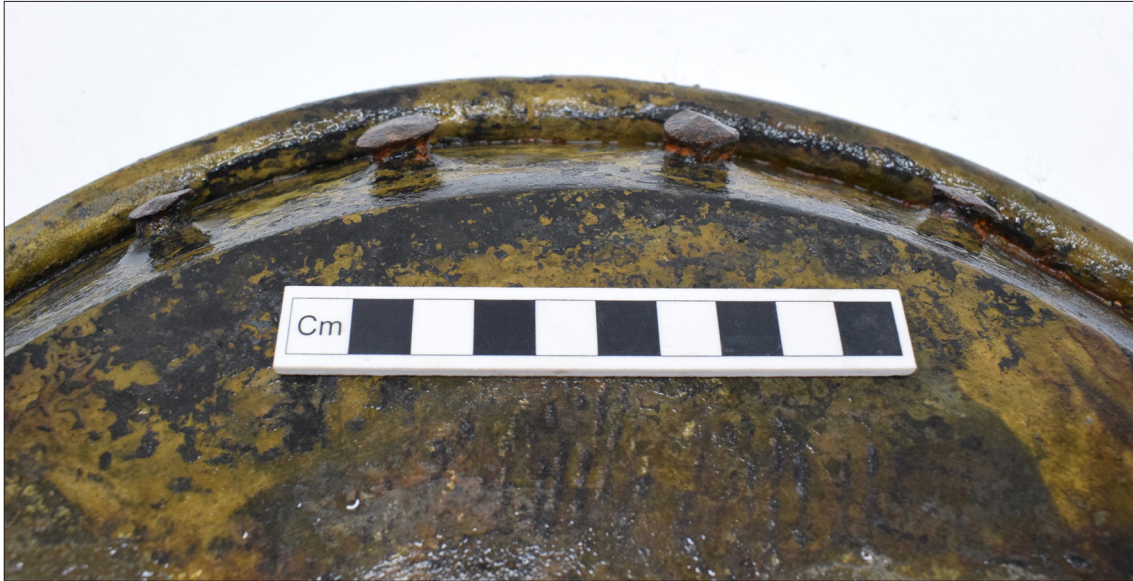
Fig 18: Object RK17 A01294 after corrosion removal showing rivets on the outside of rim.
