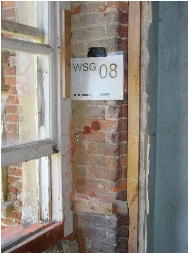
Figure 20: section of interior wall on upper floor adjacent to south-facing window showing locations WSG-08 and dosemeter below (flag D)
