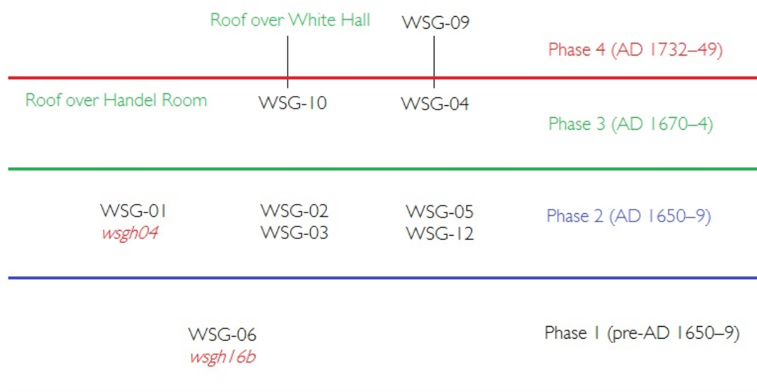
Figure 38: Diagram illustrating prior information derived from architectural, structural, and documentary evidence incorporated into the chronological model for St Giles House (black: luminescence ages; green: dendrochronology; red italic: radiocarbon wiggle-matching; solid lines indicate direct physical relationships between samples)
