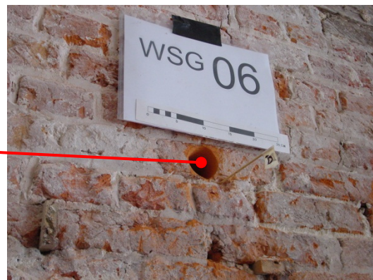
Figure 18: (a) section of north-facing interior wall of the west range adjacent to the kitchen fireplace in the basement showing location of WSG-06, (b) close-up of sampling location WSG-06 showing core hole and dosimeter (flag D)
