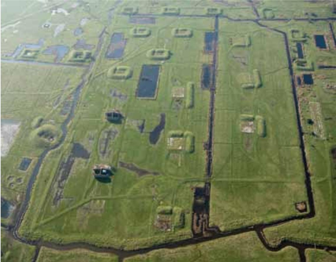
Figure 101: **Area E** viewed from the air, looking west, with cordite drying stoves in the foreground and guncotton drying stoves at the top of the image. NMR 26890/013 08-Mar-2011, Damian Grady © English Heritage.
