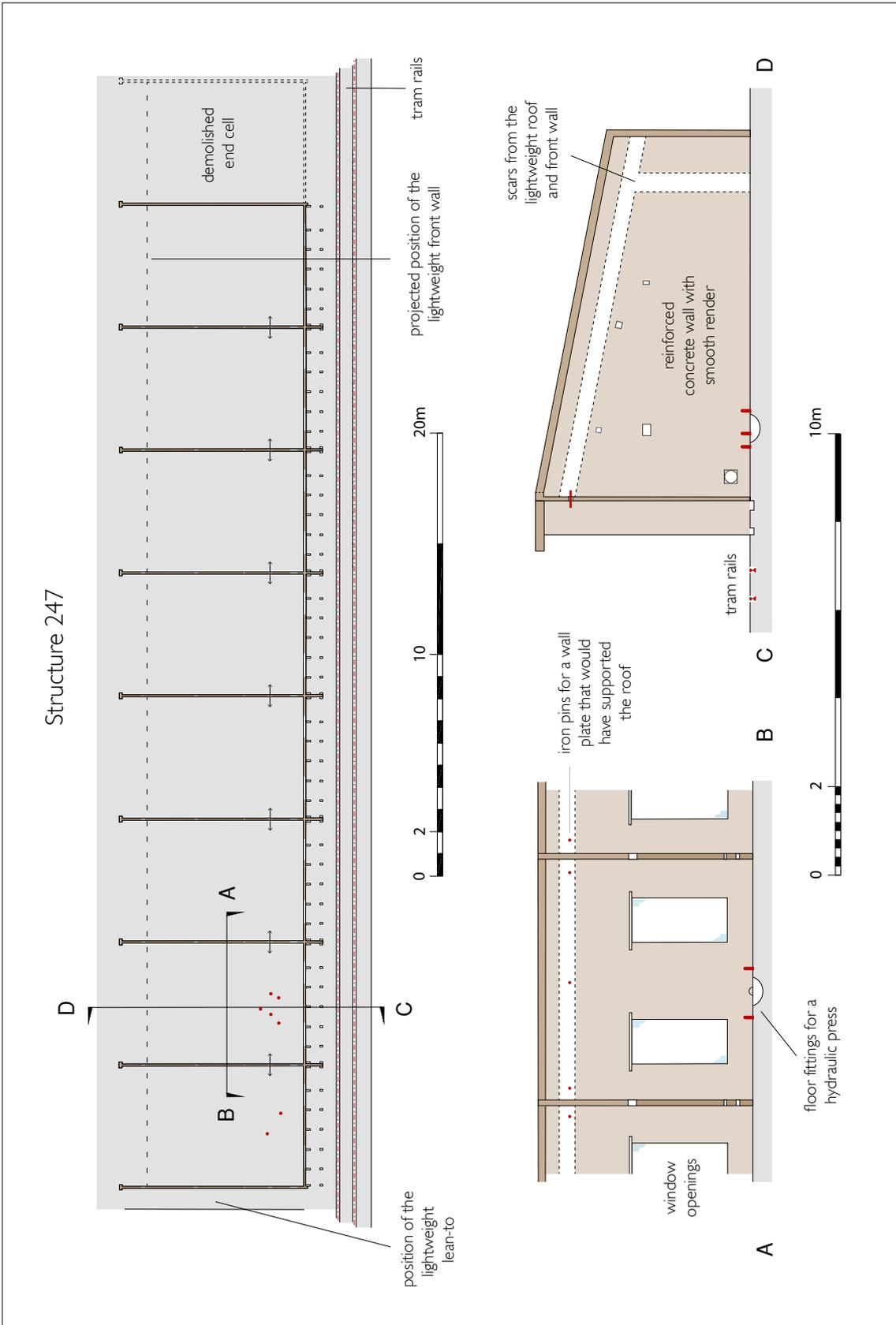
Figure 144: Schematic measured plan and section drawings of cordite press house 247. Drawn by Andrew Williams and Rebecca Pullen © English Heritage.
