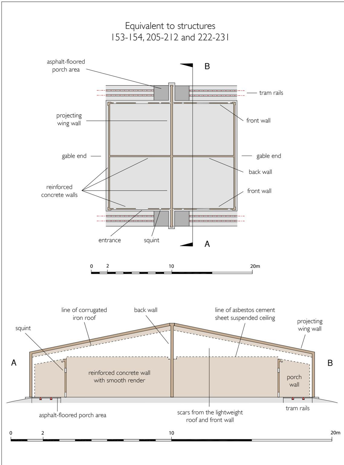
Figure 155: Schematic measured plan and section drawings of cordite drying stoves, as seen in structures **153-154, 205-212 and 222-231**. Drawn by Andrew Williams and Rebecca Pullen © English Heritage.
