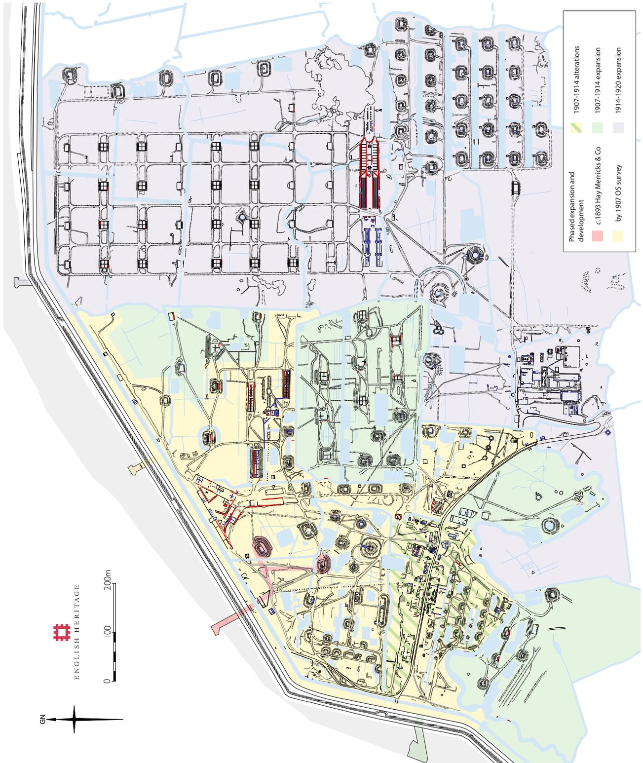
Figure 161: The main expansion and development phases of the factory. Drawn by Philip Sinton © English Heritage.
