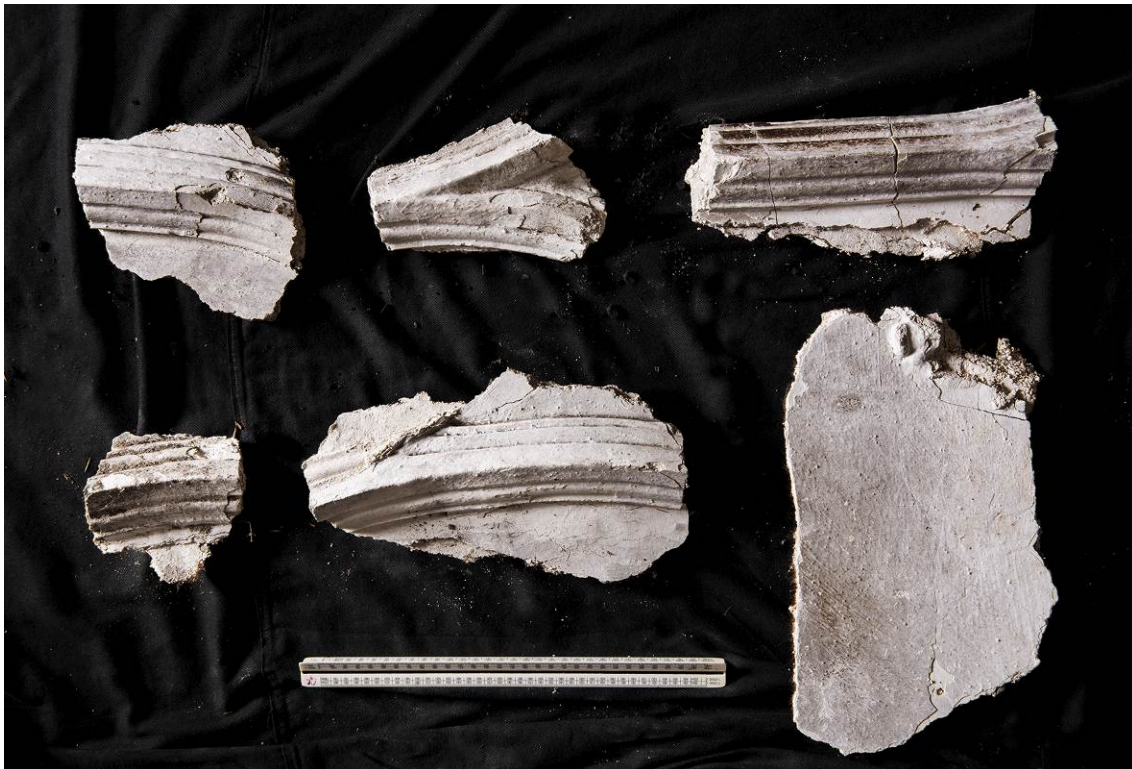
Fig 22 Fragments of plaster with single moulded ribs from the former ceiling with a 30cm scale. HEA DP196738.
