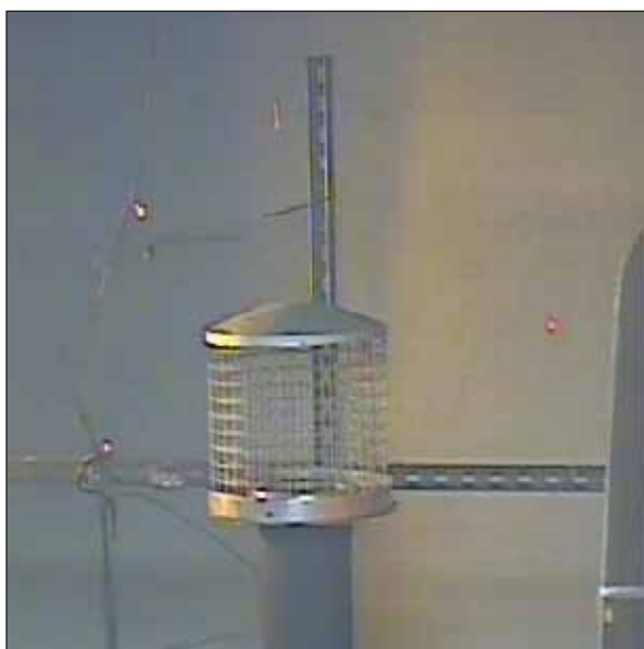
Figure 48a, b. Capped coarse mesh spark arrestor.
