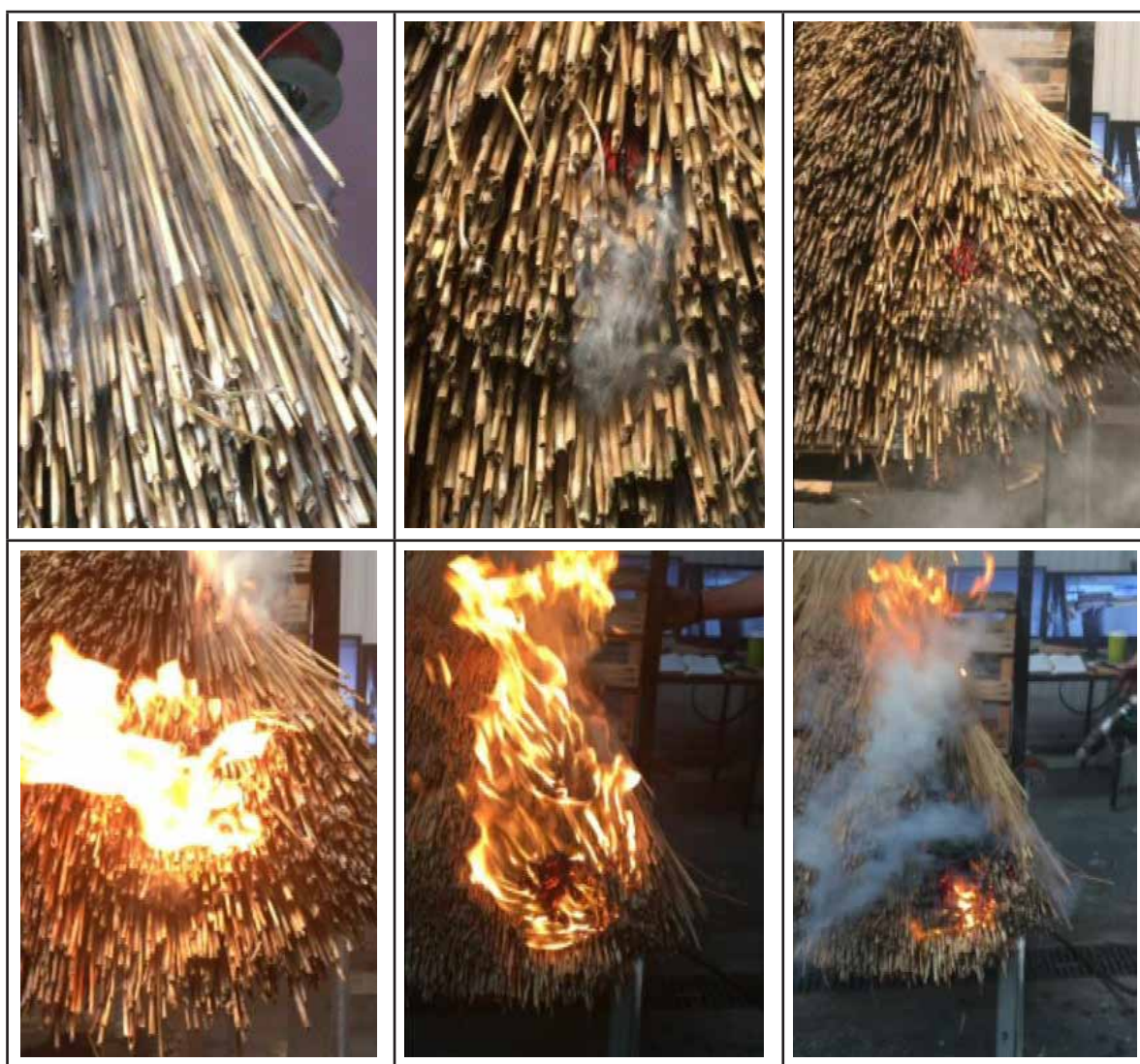
Figure 64a-f. Photo sequence of bird's nest test.
