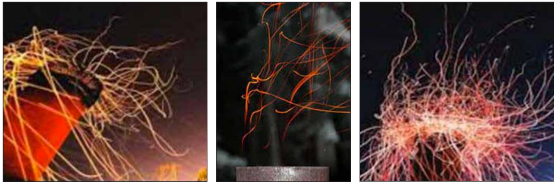
Figures 5-7. Direct spark ignition of thatch.
