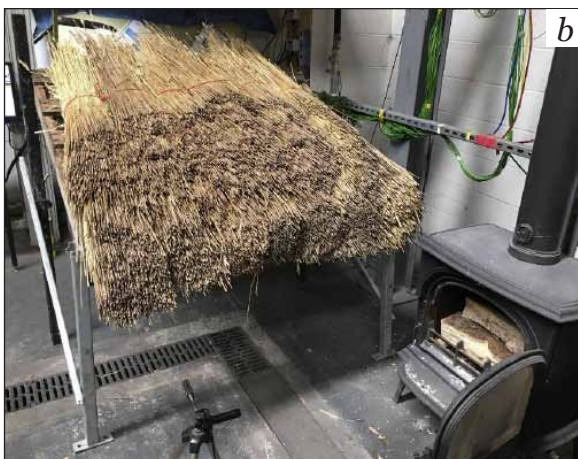
Figure 63a, b. Bird's nest hazard simulation with thatch below.
