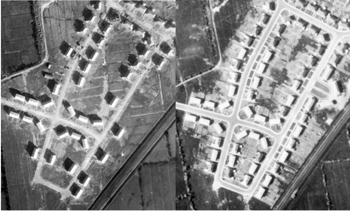
Figure 43 Bournville East in 1948 and 1950. Gaps between houses in 1948 filled with Cornish Units by 1950. Details of RAF/CPE/UK/2489 V5011 11-MAR-1948 and RAF/541/527 RP 3245 14-MAY-1950 Historic England Archive (RAF Photography)
