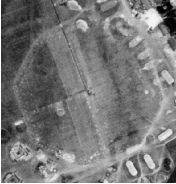
Figure 77 The outline of Uphill HAA's octagonal GL mat. Detail of RAF/GHQ/105 V 14-MAY-1941 Historic England Archive (RAF Photography)
