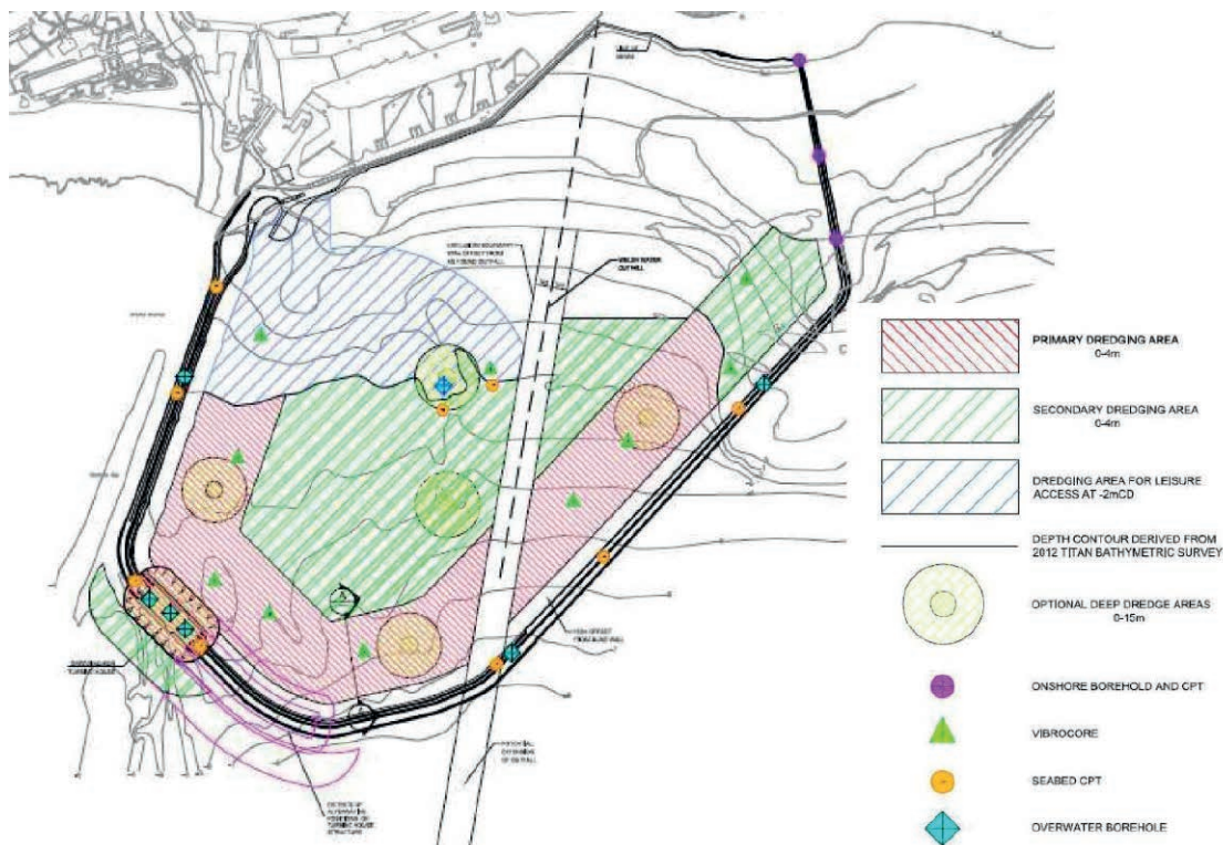
Fig 1 Proposed dredging plan within Swansea Bay Tidal Lagoon impoundment (Tidal Lagoon Swansea Bay, 2014).
