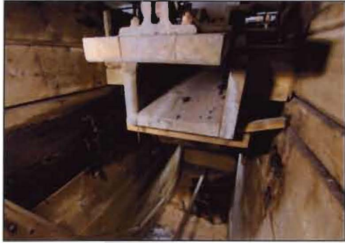
Figure 59. Mechanism for agitating cloth inside a milling machine. [DP043864]
