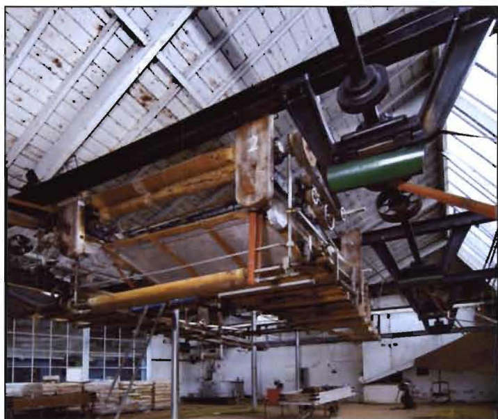
Figure 60. One of the portable sewing machines used for stitching cloth pieces. [DP043861]
