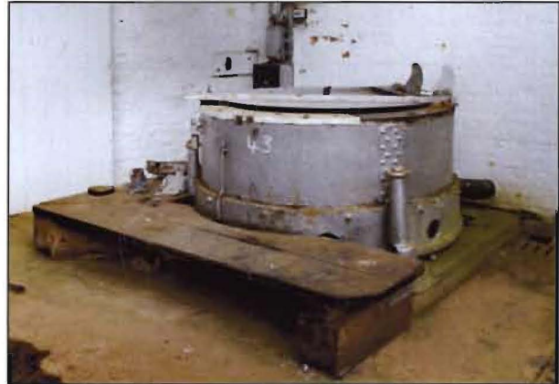
Figure 57. One of the two centrifuge drying machines [DP043916]
