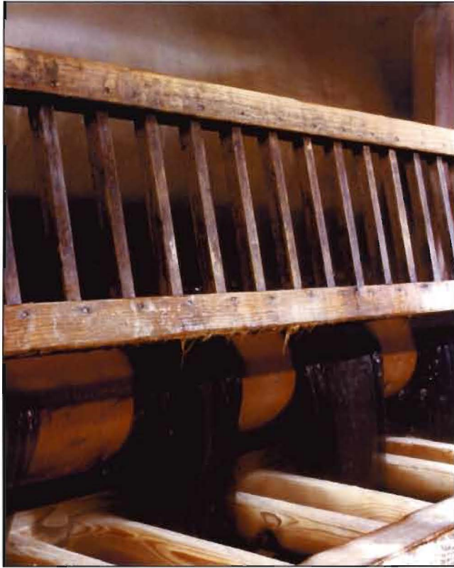
Figure 18. Three cloth pieces being scoured at Tone Works in 1995. [AA96/00664]
