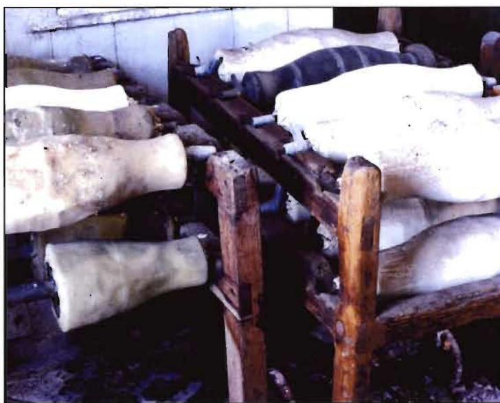
Figure 4. Disused equipment used for moulding Fox's Patented Improved Puttees, photographed at Tonedale in 1995.[AA96/03915]
