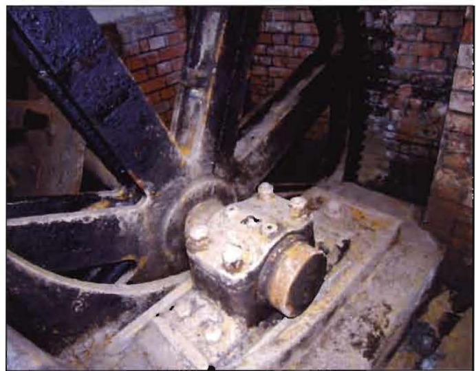
Figure 40. Detail of the gear chamber, showing the main spur gear mounted on the pinion shaft. [DP046036]
