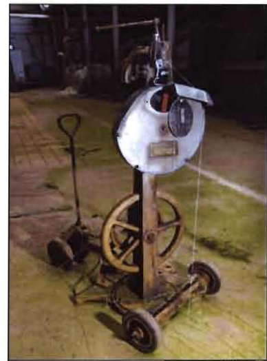
Figure 60. One of the portable sewing machines used for stitching cloth pieces. [DP043861]
