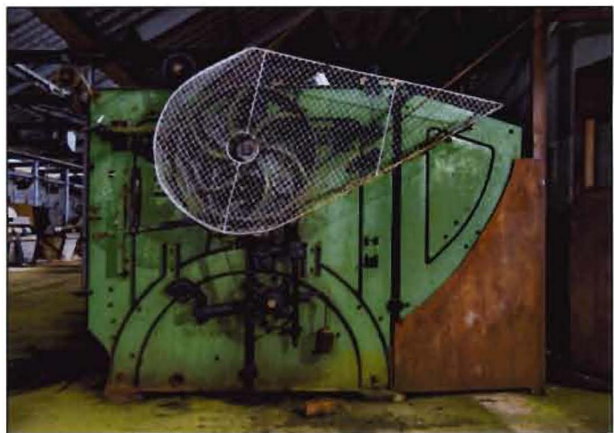
No 32. Milling machine, early or mid-20 th century, by Hemmer of Aachen. Solid cast-iron sides (similar to 21). Driven by a clutch pulley. [DP043891]
