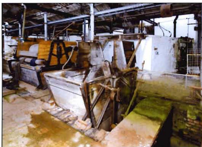
No 8. Combined milling and scouring machine, mid-20 th century, similar to 5, 6 and 7, and partly dismantled. [DP043841]
