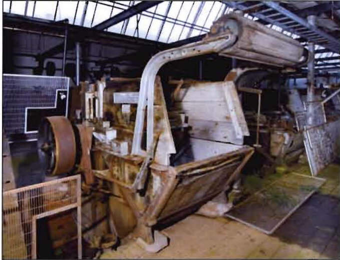
No 6. Combined milling and scouring machine, mid-20 th century with later alterations, by John Mitchell & Sons Ltd., Brockholes. Wooden construction on a cast-iron frame. Patent on name plate (409869) refers to a 1934 system for controlling milling rollers. [DP043834]
