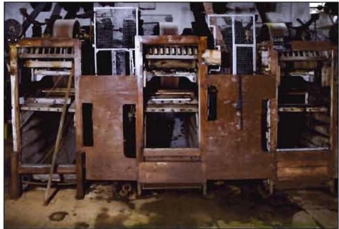
Nos 30-31. Milling machines, mid-20 th century, maker not known, wooden construction on a cast-iron frame. Driven by a clutch pulley. [DP043886]
