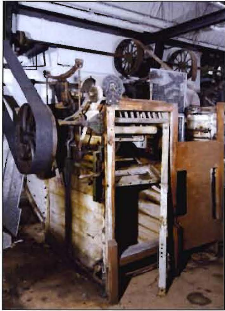
No 29. Milling machine, mid-20 th century, maker not known. Similar features to others but slightly longer in plan. Driven by a clutch pulley. [DP043884]
