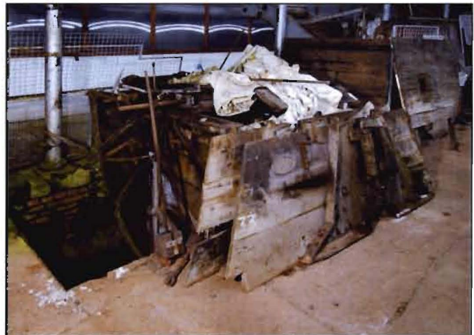
No 7. Combined milling and scouring machine, mid-20 th century, similar to machines 5 and 6 but partly dismantled. John Mitchell and Sons, Brockholes, Huddersfield. Clutch pulley drive. [DP043840]
