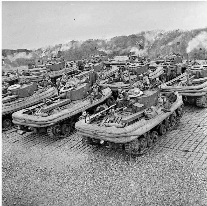
Figure 8. Valentine tanks, with modifications for amphibious landings, on one of the Stokes Bay Hards (copyright Imperial War Museum, H 35177).
