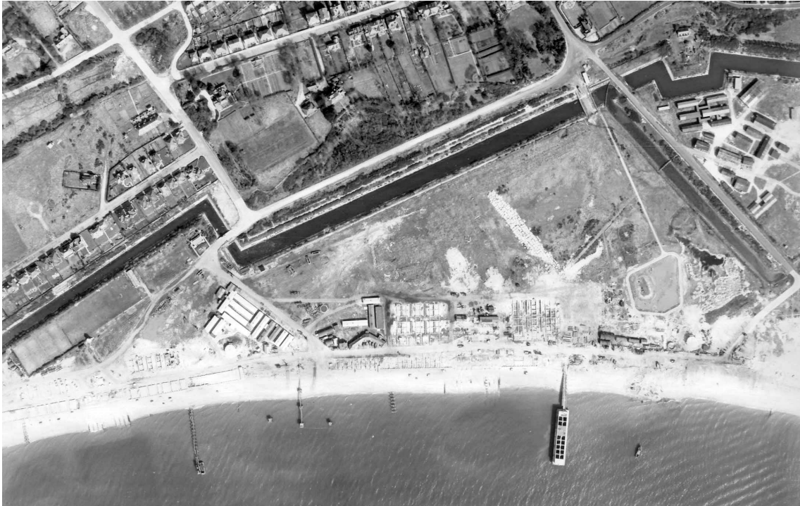
Figure 56. Approximately the same area as figure 55 in March 1946. Mooring dolphins associated with embarkation hards G3 and G4 are clearly visible in the water and on the beach. Phoenix caisson construction sites 1 and 2 are immediately behind the beach. The hatted encampment associated with Gilkicker Heavy Anti-Aircraft Battery is visible on the right of the image. Pre-war features include the bathing pool and associated paths on the right of the image and the still water-filled Stokes Bay Lines zig-zagging from left to right across the centre of the image. RAF/106G/UK/1322 V 5025 28-MAR-46, Historic England Archive (RAF Photography).
