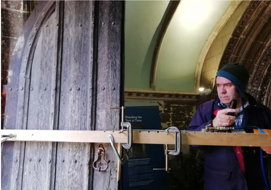
Figure 7: Coring of the north door leaf with Dan Miles using the micro-borer and jig which allows the coring bit to pass through successive boards within the thickness of the board (photograph Martin Bridge)
