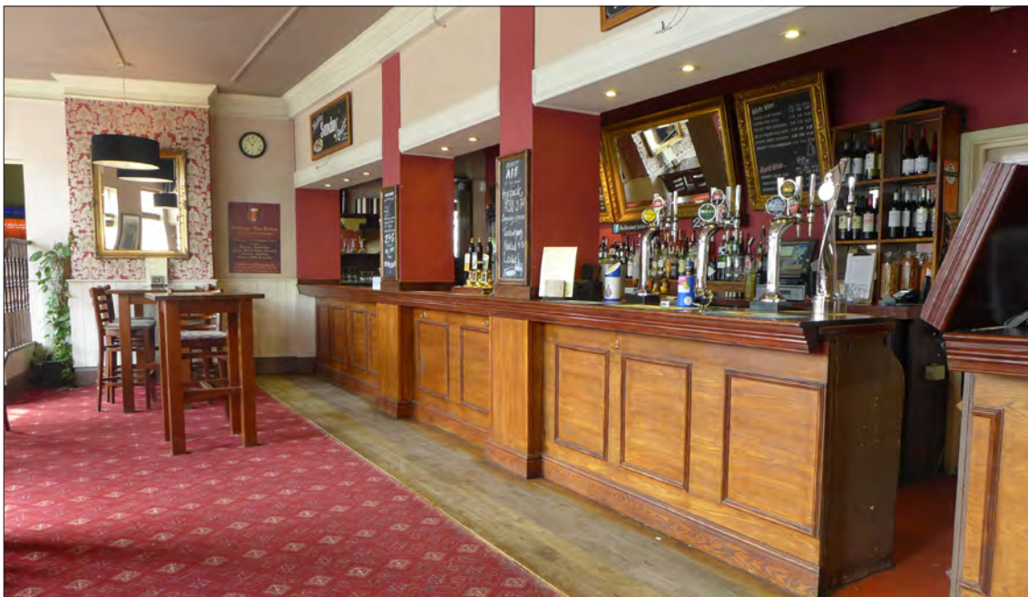
2.6 A pub which has been internally altered is the Berrylands Hotel, Surbiton, London, designed by Joseph Hill for Hodgson's Kingston Brewery and built in c. 1934. This counter at the centre of the pub occupies the site of an earlier servery which opened onto three separate spaces – a private bar and a ladies' bar, divided by an off sales compartment – the former divisions of which are marked by the piers. (© Historic England, Emily Cole)
