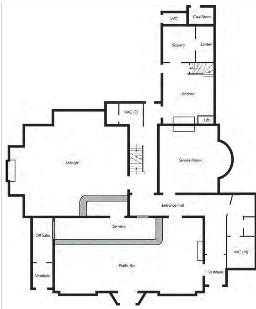
12.6.2 The ground-floor plan of the Biggin Hall Hotel, based on that produced by the pub's architect, T. F. Tickner, in c. 1921. (© Historic England, Philip Sinton)
