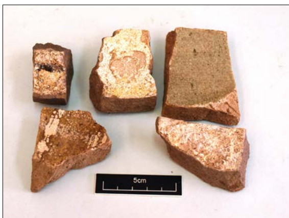
Fig 10: Crucible fragments from Lordings Farm (interior surfaces) (context [102])
