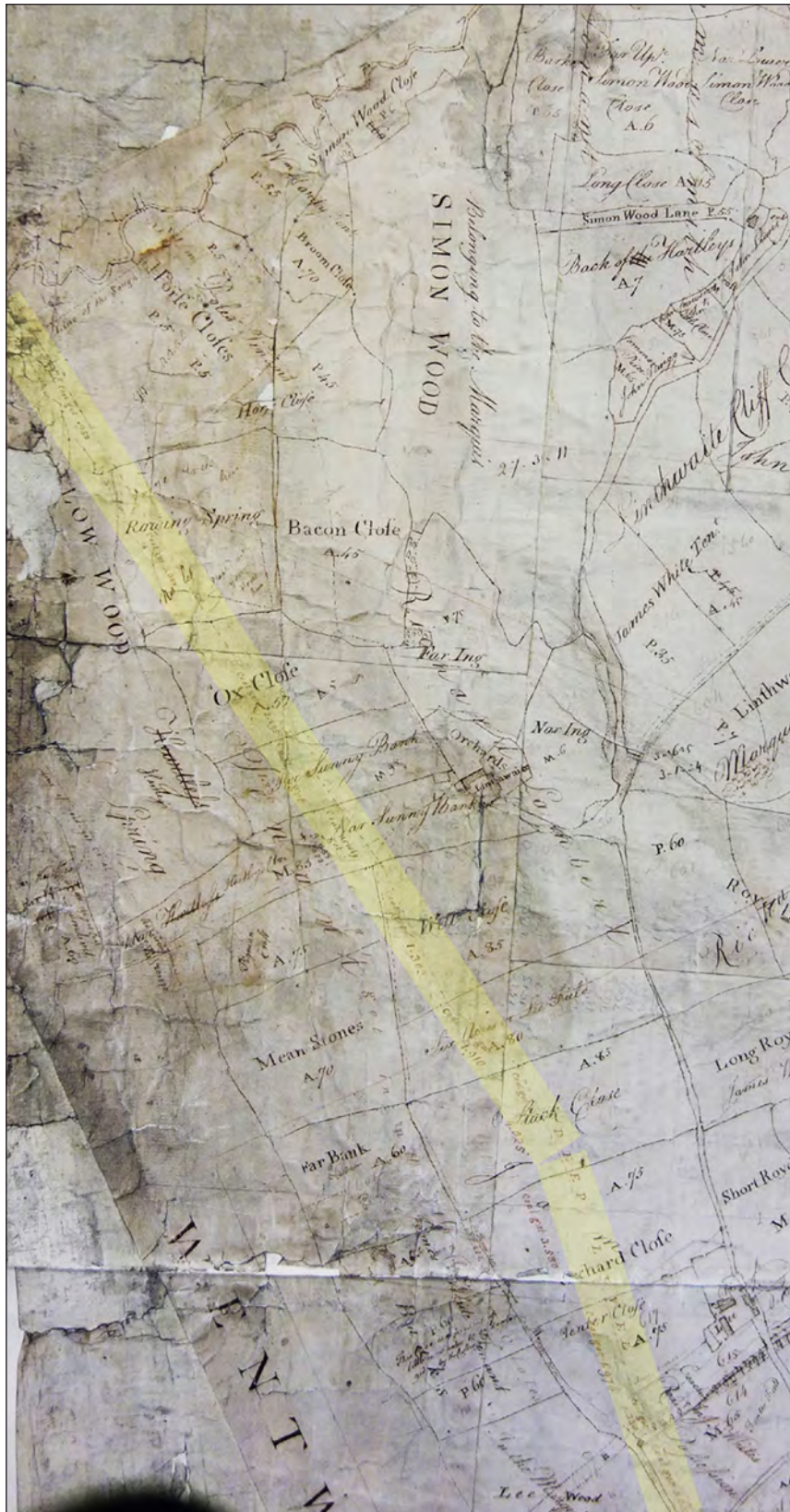
Fig 8. Extract from the Draft Brampton Bierlow Township Plan 1773, showing (highlight added) the line of Lowwood Colliery deep level and sough. North is to the top. Reproduced courtesy of Sheffield City Archives, FC/P/Wath/4L.
