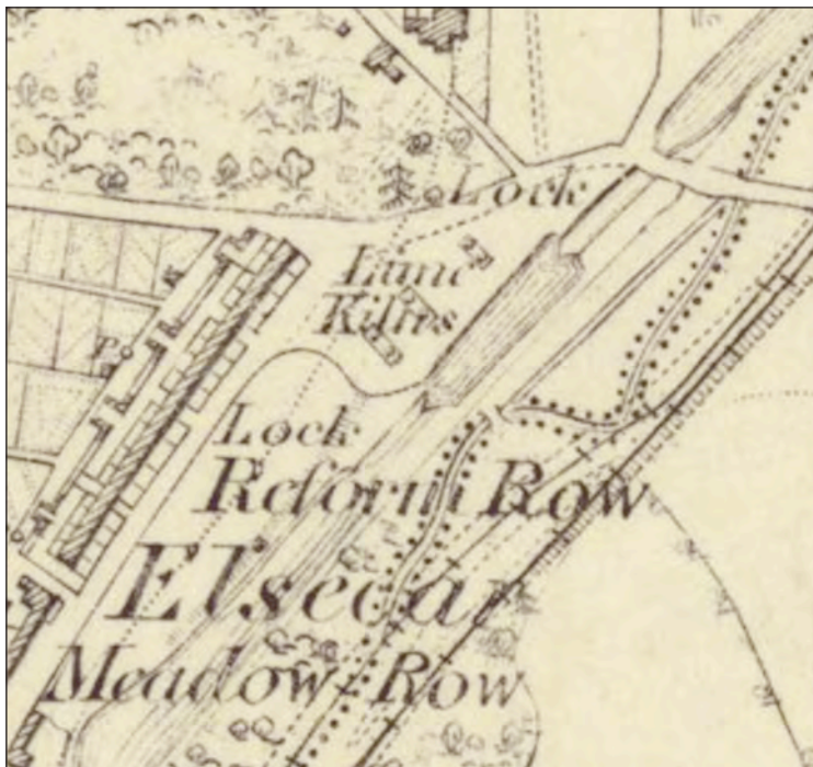
Fig 186. Extract from the 1st edition Ordnance Survey 6-inch map, sheet 283, 1855 (surveyed 1849-50) showing the three banks of lime kilns, each seemingly with two charging holes indicating twin furnaces. Reproduced with permission from the National Library of Scotland.
