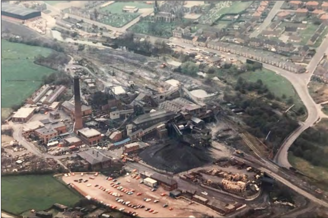
Fig 27. Aerial photograph of Elsecar Main Colliery, taken before the site closed. The car park and coal stack can be seen in the foreground. The chimney, winding gear and coal preparation plant are visible at the centre of the complex. Aligned in parallel with the canal are a series of slurry settling beds. Reproduced with the kind permission of Barnsley Archives and Local Studies.
