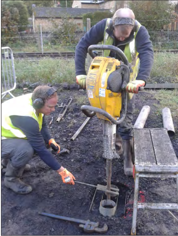
Fig 72. Quaternary Scientific (Reading University) staff engaged in the bore-hole survey, October 2018. © Barnsley Museums, T Roberts.
