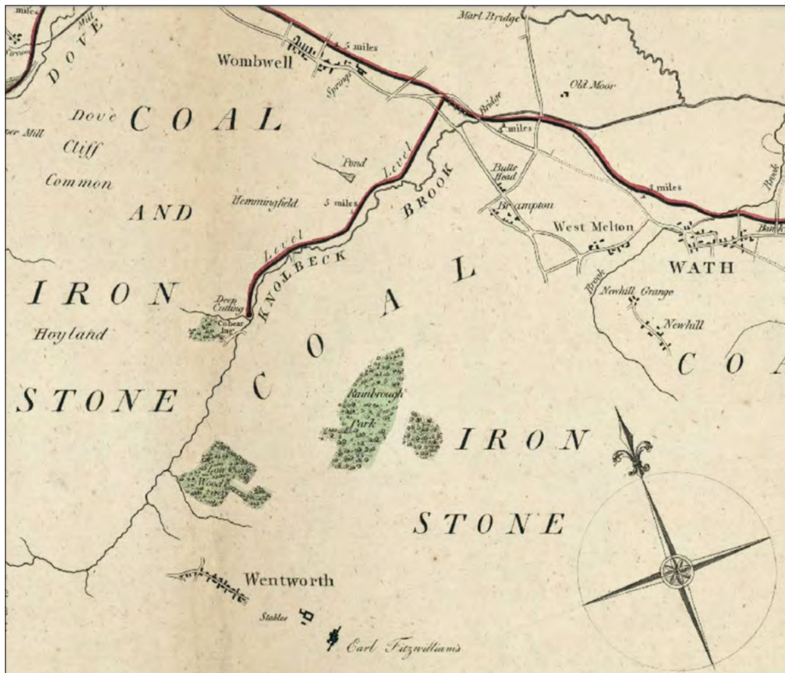
Fig 12. Extract from 'A Plan of the intended Dearn and Dove Canal: describing the Branches from it with the adjacent Rivers & Brooks.' John Thompson, Engineer and William Fairbank, Surveyor. 1793. The intended line of the canal is shown in red. Reproduced with permission from Sheffield Archives, X466.
