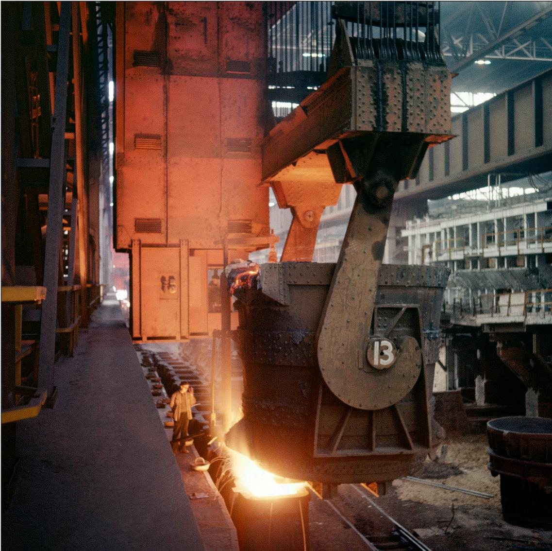
Figure 6. Casting steel ingots at Port Talbot, c1970 (FF98\_00246, Historic England Archive).
