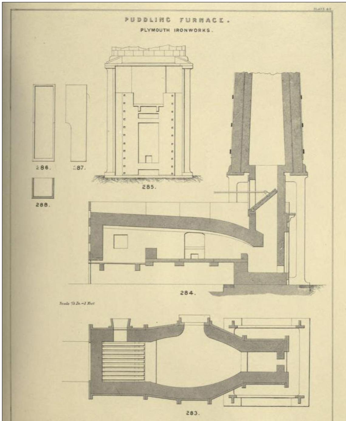
Figure 3. Mid-19<sup>th</sup> century puddling furnace (Truran 1862, Plate 49)
