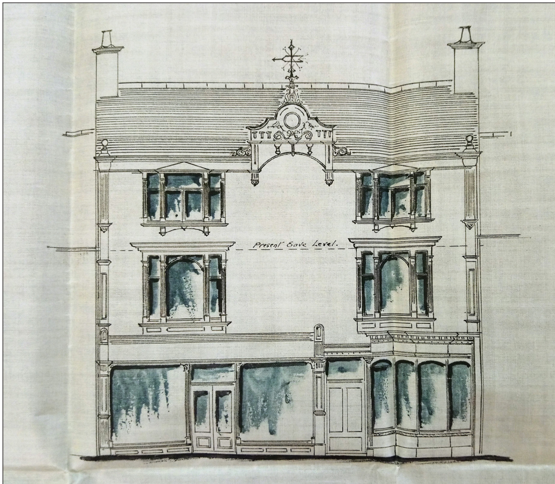
Figure 6: Proposed elevation of 25 Newgate Street with second-floor extension, designed by R B Thompson, 1909 (UD/BA 432/1206 Bishop Auckland Urban District Council. Reproduced with permission of Durham County Record Office)
