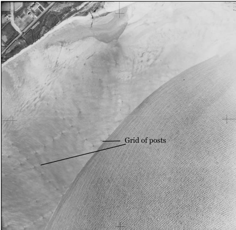
Figure 46: Second World War anti-invasion defences on the mud flats of Pegwell Bay made up of an extensive grid of posts or stakes exposed at low tide. Extract from RAF/HLA/540/V/6053 17-MAY-1942 Historic England Archive (RAF Photography).
