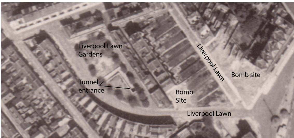
Figure 47: The Second World War public air raid shelter tunnel entrance visible as an L-shaped access in Liverpool Lawn Gardens, Ramsgate in May 1942. This was later in-filled and capped, and is now invisible beneath the grass. Extract from RAF/HLA/540/V/6094 17-MAY-1942 Historic England Archive (RAF Photography).
