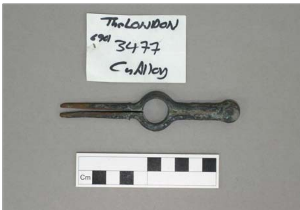
Fig 15: SF3477: Navigational dividers. Double-handed straight dividers. Straight truncated pyramidal-sectioned arms (forming octagonal shape when closed) each with arched middle forming open circle when dividers are closed; profiled scroll below arches. Arms of equal length, section below circle has higher triangular shape than above; tips both with intentional (L1 5.4mm, L2 4.8mm) split. Hinged end double conical ball-shaped with flat equator.
