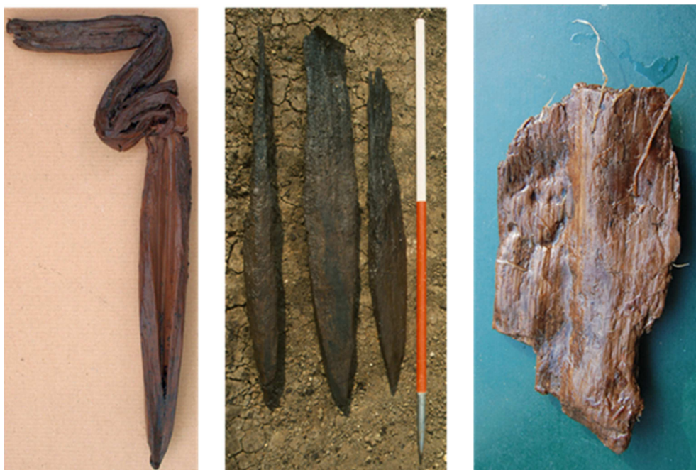
Figure 2: Left: Image of an upright wall post excavated from Glastonbury Lake Village, displaying the 'dog-leg' kink caused by peat shrinkage. Centre: Timber excavated from a Middle Saxon bridge near Glastonbury, exhibiting the characteristic pointed tops caused by preferential decay of the sapwood in parts of the timbers located above the waterlogged zone. Right: Root damage in a wood chip from Glastonbury Lake Village, caused when wood is weakened such that roots can penetrate through it. Images courtesy of Richard Brunning, copyright South West Heritage Trust.
