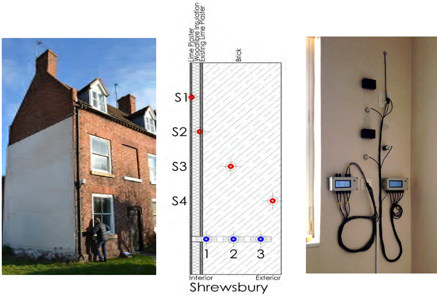
Figure 2. Interstitial hygrothermal gradient and material moisture monitoring, Abbeyforegate, Shrewsbury 2014.
