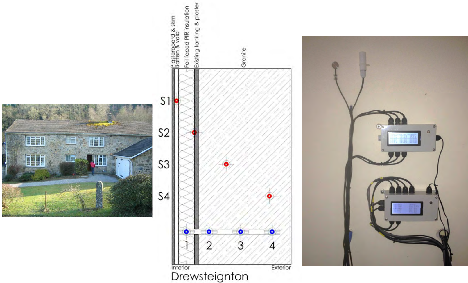
Figure 3. Interstitial hygrothermal gradient and material moisture monitoring, Drewsteignton, 2014.
