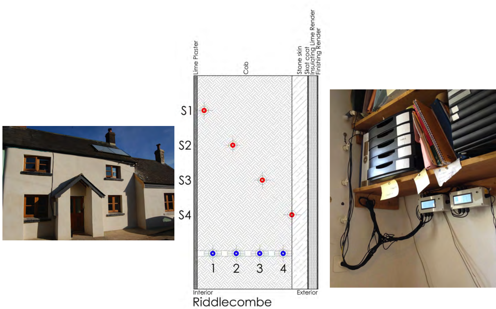
Figure 4. Interstitial hygrothermal gradient and material moisture monitoring, Riddlecombe.
