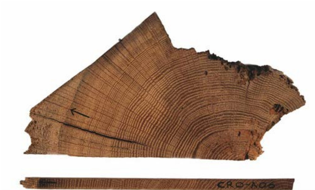
Figure A1.2: Cross-section of a rafter, showing sapwood rings in the left-hand corner, the arrow points to the heartwood/sapwood boundary (H/S); and a core with sapwood; again the arrow is pointing to the H/S. The core is about the size of a pencil
