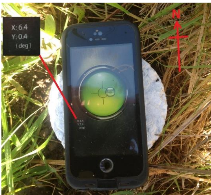
Figure 8. Photograph of the Surface app in use on top of one of the concrete cylinders. Inset: angles measured in x (west-east) and y (north-south) planes
