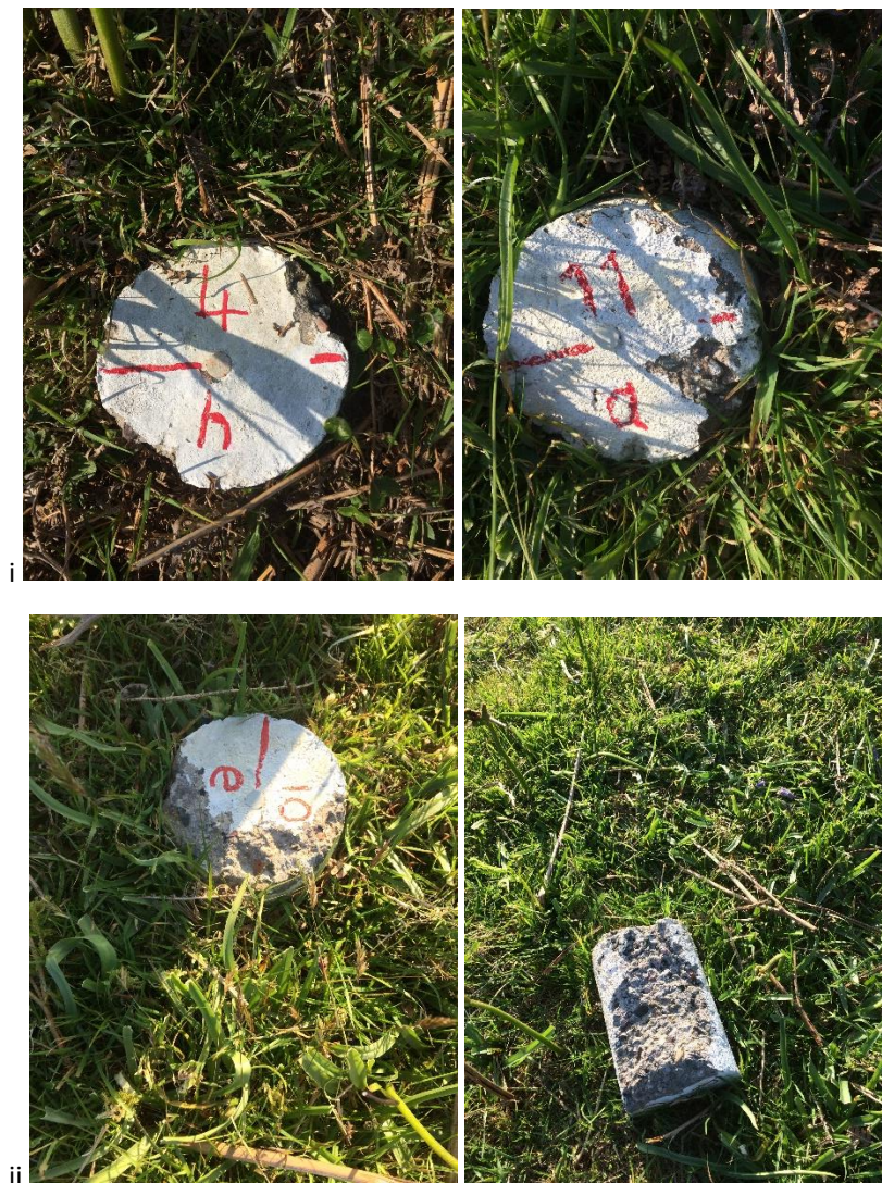
Figure 73. Examples of physical damage to cylinders at Challacombe Farm, following (i) bashing & (ii) cutting in 2016
