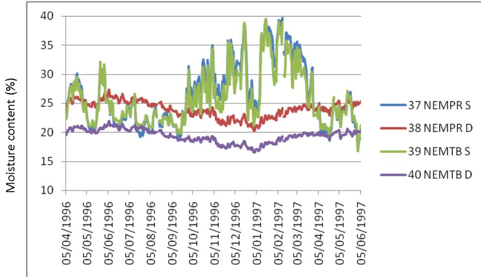
Graph 55: Surface and deep moisture content readings from tie beam and principal rafter at mid height N eaves
