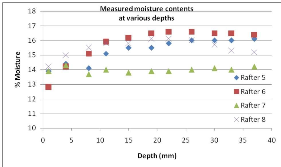
Graph 78a: Moisture content readings at various depths in rafters 5 to 8
