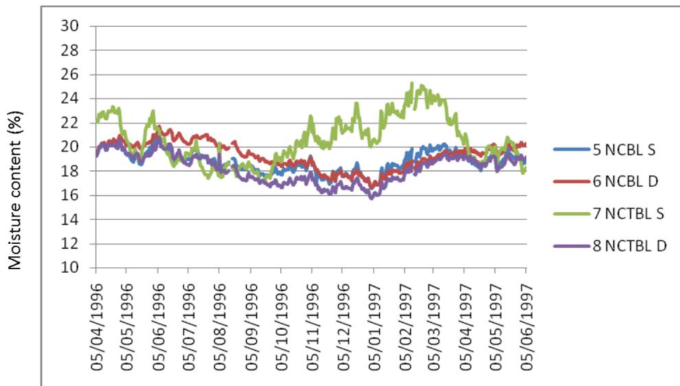
Graph 47: Surface and deep moisture content readings from the Nave central beam and tie beam
