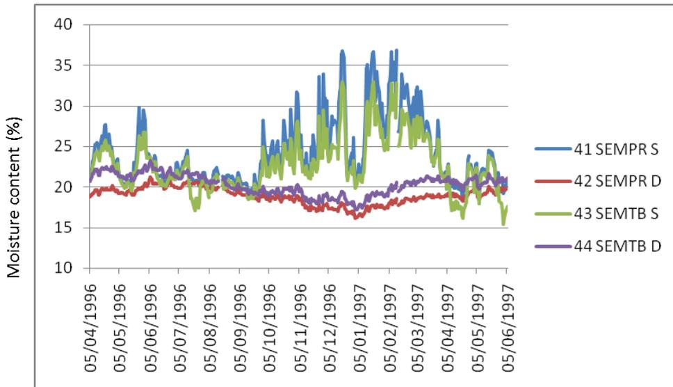
Graph 56: Surface and deep moisture content readings from tie beam and principal rafter at mid height S eaves
