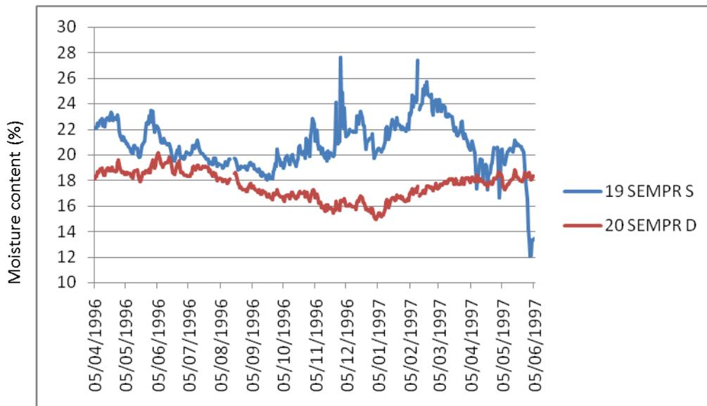
Graph 52: Surface and deep moisture content readings from the principal rafter at mid height in the S eaves
