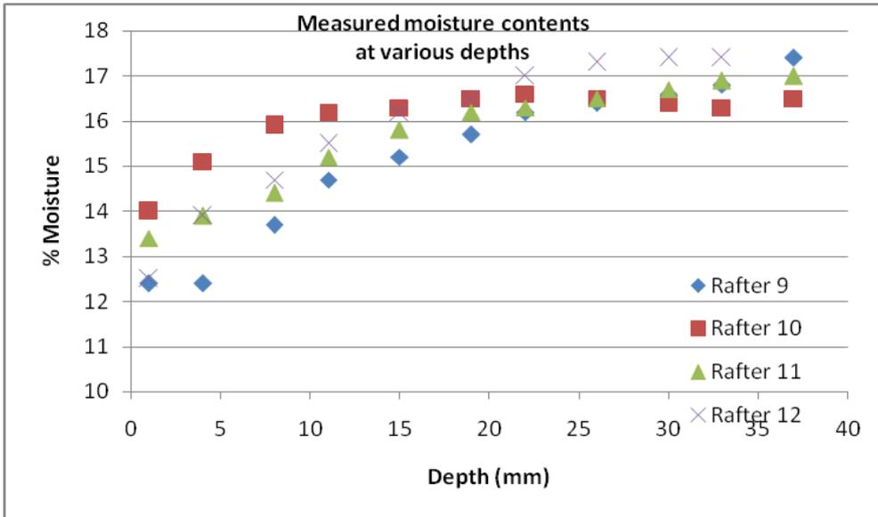
Graph 79: Moisture content readings at various depths in rafters 9 to 12
