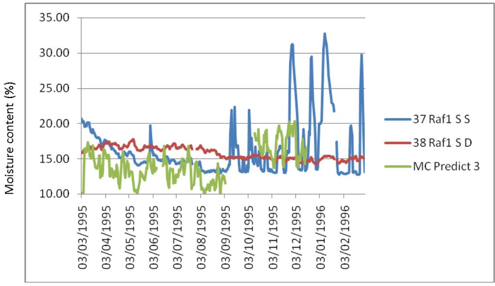
Graph 67: Winchester Cathedral: Surface and deep moisture content readings from old oak rafter at eaves level compared with predicted moisture content
