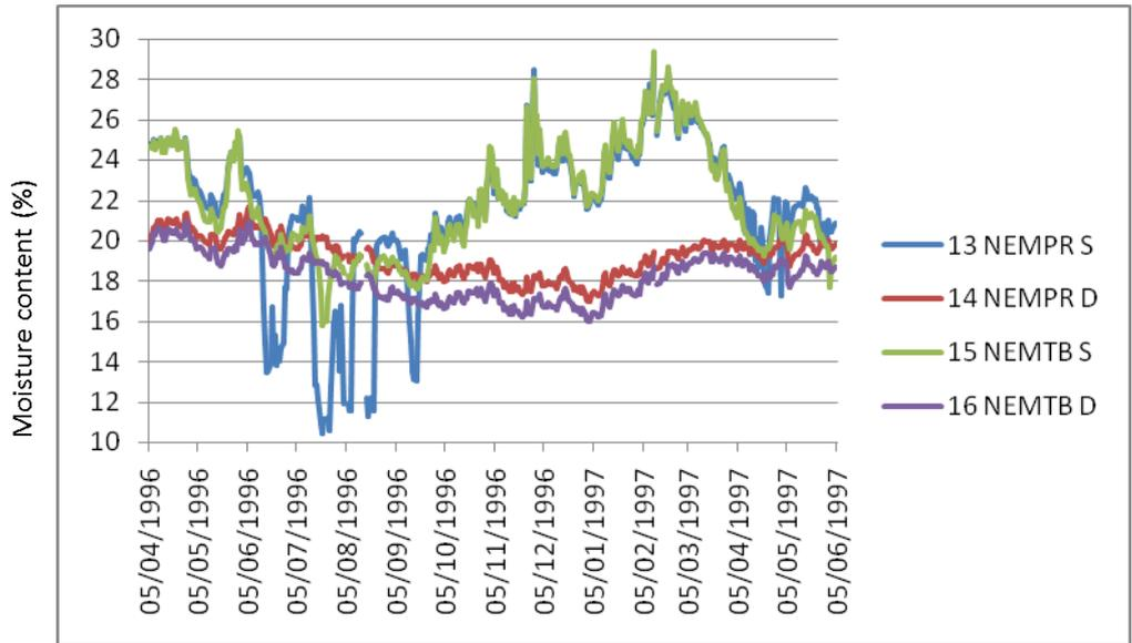
Graph 49: Surface and deep moisture content readings from principal rafter and tie beam at N eaves
