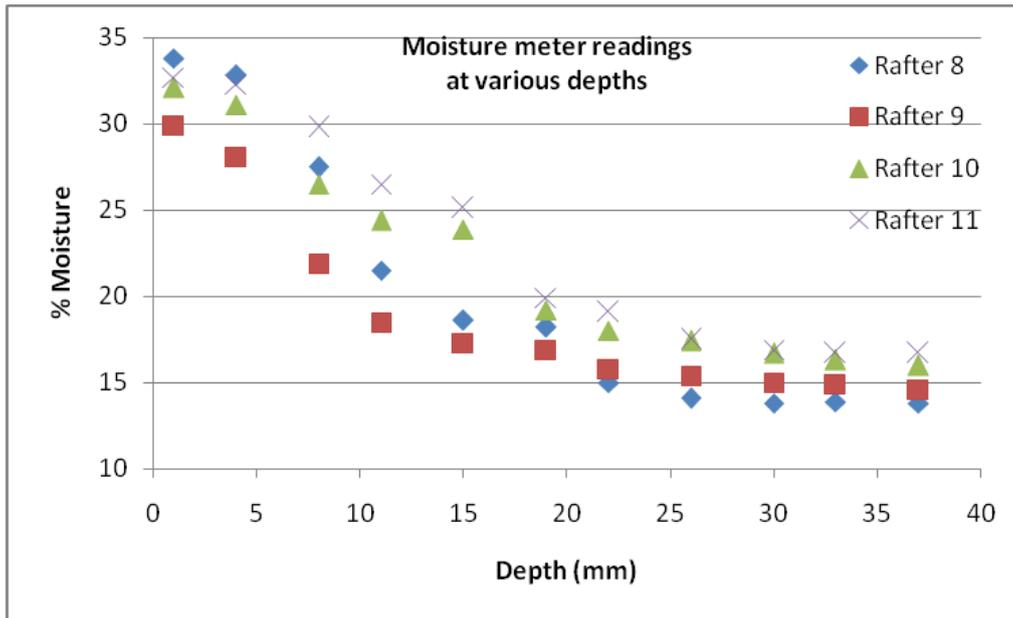
Graph 77: Moisture content readings at various depths in rafters 8 to 11
