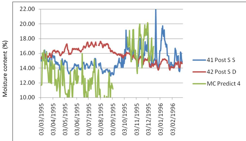
*Graph 66: Winchester Cathedral: Surface and deep moisture content readings from old oak post in centre of roof compared with predicted moisture content*
