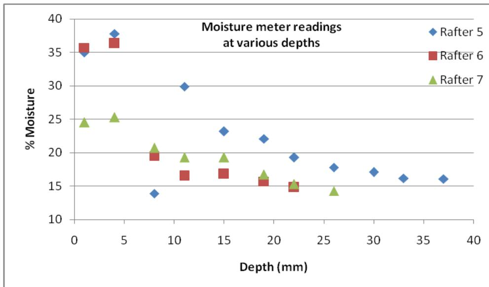
Graph 76: Moisture content readings at various depths in rafters 5 to 7
