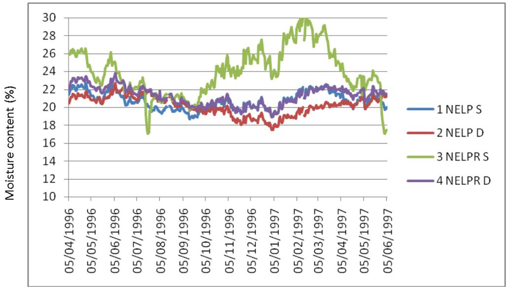
Graph 45: Surface and deep moisture content readings from timbers at N eaves in Nave
