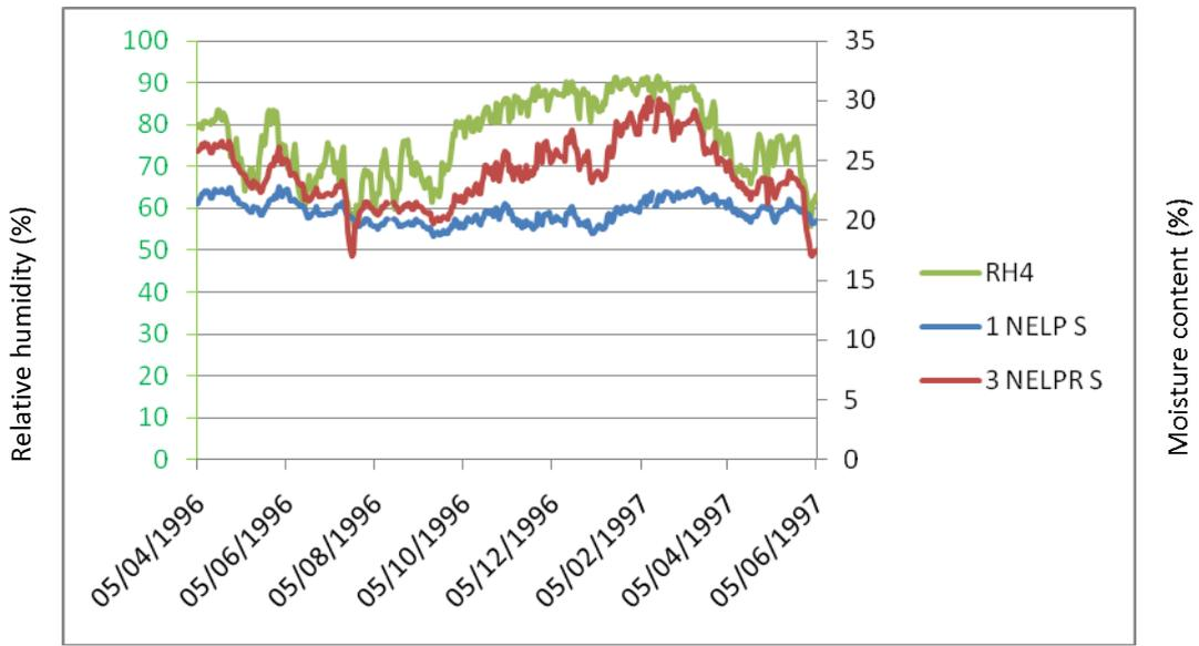
Graph 46: Surface moisture content readings from plate and rafter at N eaves compared with relative humidity
