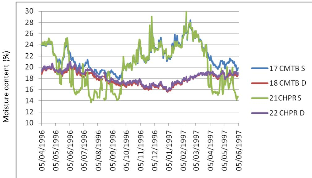
Graph 51: Surface and deep moisture content readings from tie beam and principal rafter
