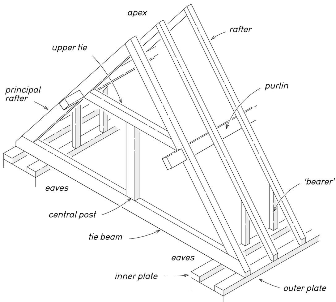
Figure 1: Terms used in this report to describe roofing timbers
