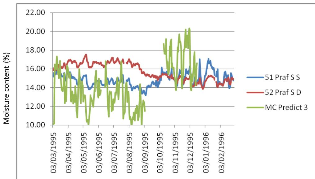
Graph 70: Winchester Cathedral: Surface and deep moisture content readings from medieval oak principal rafter on S side of roof compared with predicted moisture content
