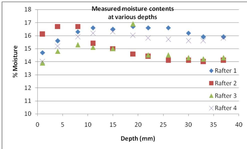
Graph 78: Moisture content readings at various depths in rafters 1 to 4
