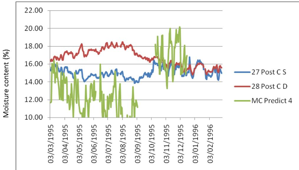
Graph 69: Winchester Cathedral: Surface and deep moisture content readings from medieval oak in centre of roof compared with predicted moisture content
