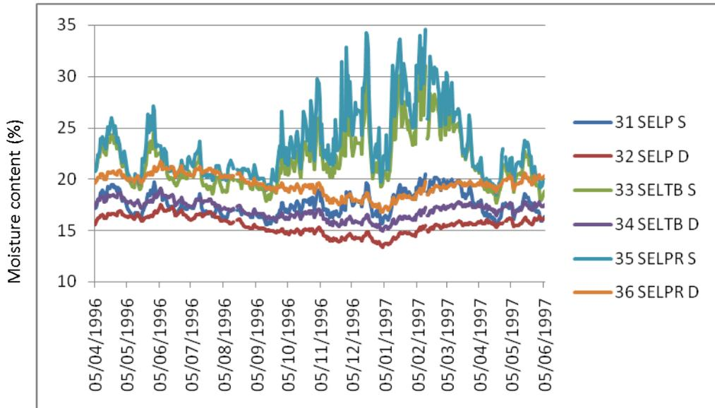
Graph 54: Surface and deep moisture content readings from plate, tie beam and principal rafter at S eaves
