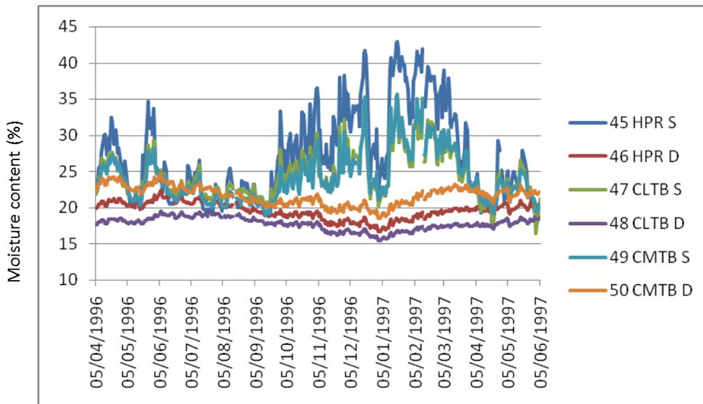
Graph 57: Surface and deep moisture content principal rafter, tie beam and mid-level tie
