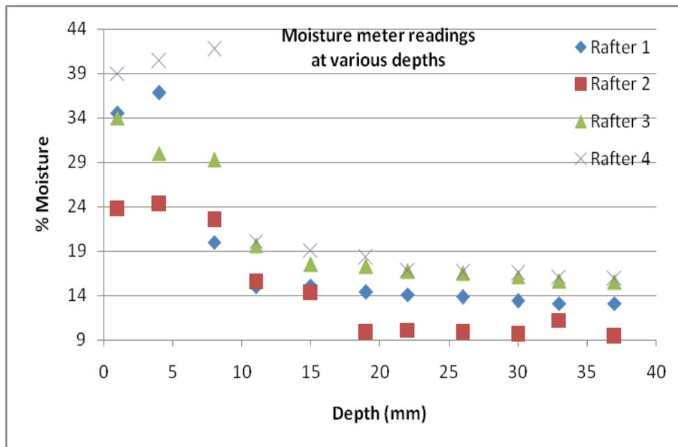
Graph 75: Moisture content readings at various depths in rafters 1 to 4
