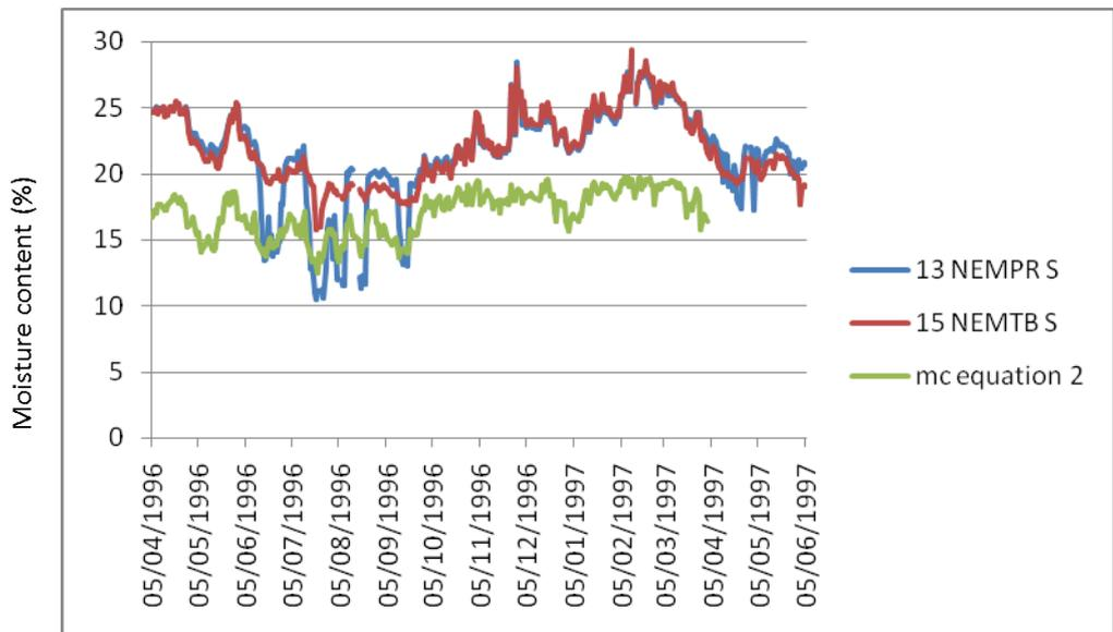
Graph 50: Surface and deep moisture content readings from tie beam and principal rafter at N eaves compared with calculated equilibrium moisture content using the Hailwood Horrobin equation (Equation 2)
