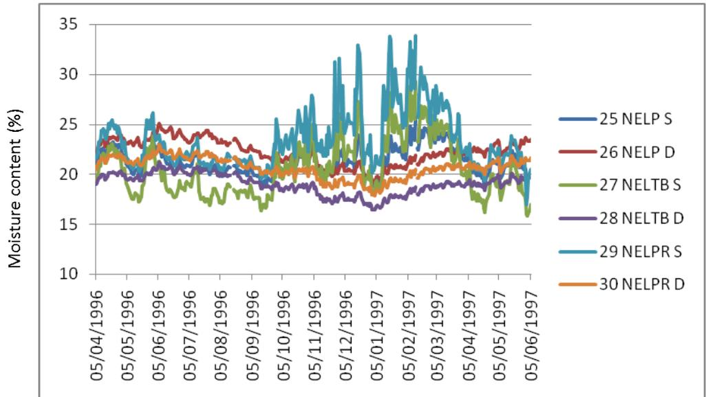
Graph 53: Surface and deep moisture content readings from plate, tie beam and principal rafter at N eaves
