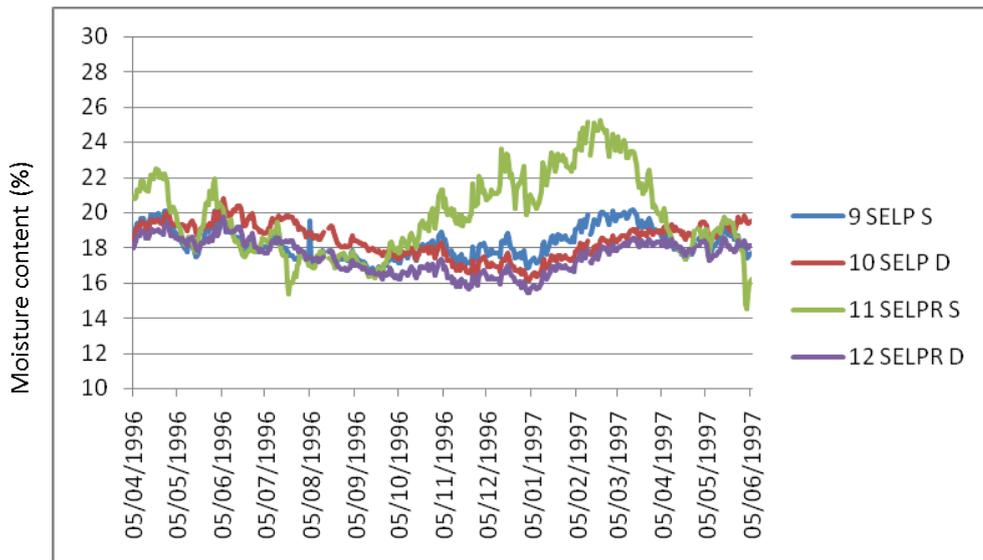
Graph 48: Surface and deep moisture content readings from plate and principal rafter at S eaves
