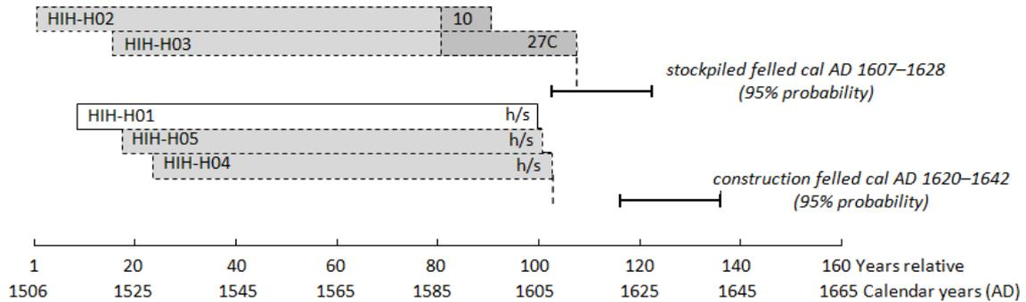
Figure 9: Summary diagram showing the dated timbers from the roof of Higham House (date ranges for felling episodes derive from the model defined in Figure 7)
