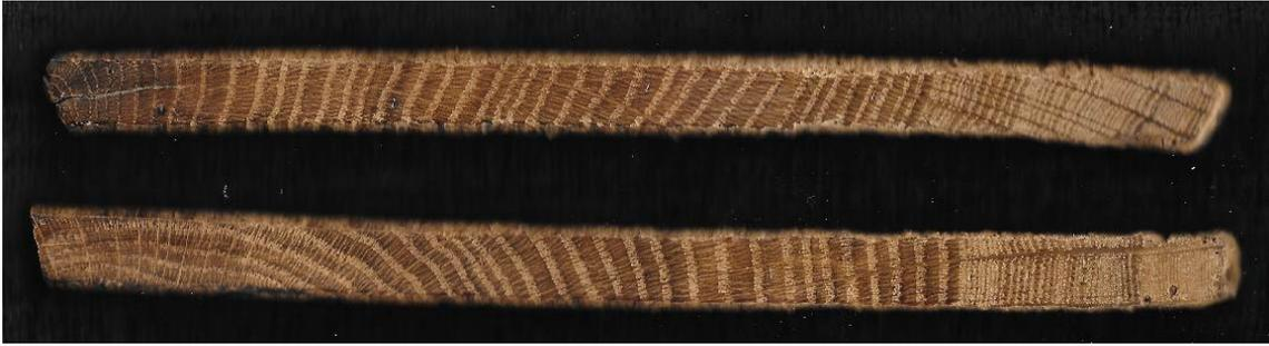
Figure 5: The cores from the principal rafters, HIH-H02 (top) and HIH-H03 (bottom), showing the abrupt growth changes and the clear lack of recovery to previous growth levels throughout the latter years of growth of the tree from which HIH-H03 was derived (photograph Robert Howard)
