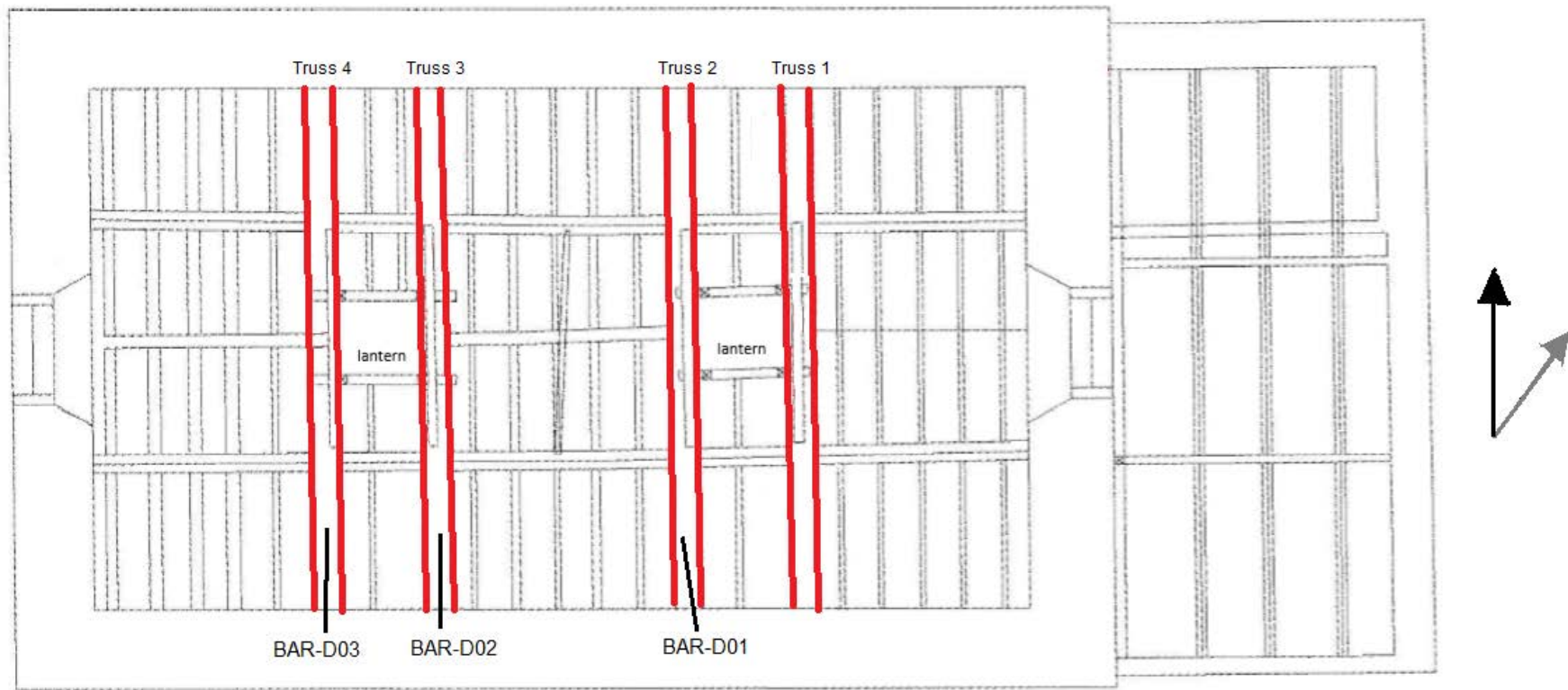
Figure 8: Plan of the dovecote, showing the location of sampled timbers BAR-D01–3 (after Archaeological Project Services)
