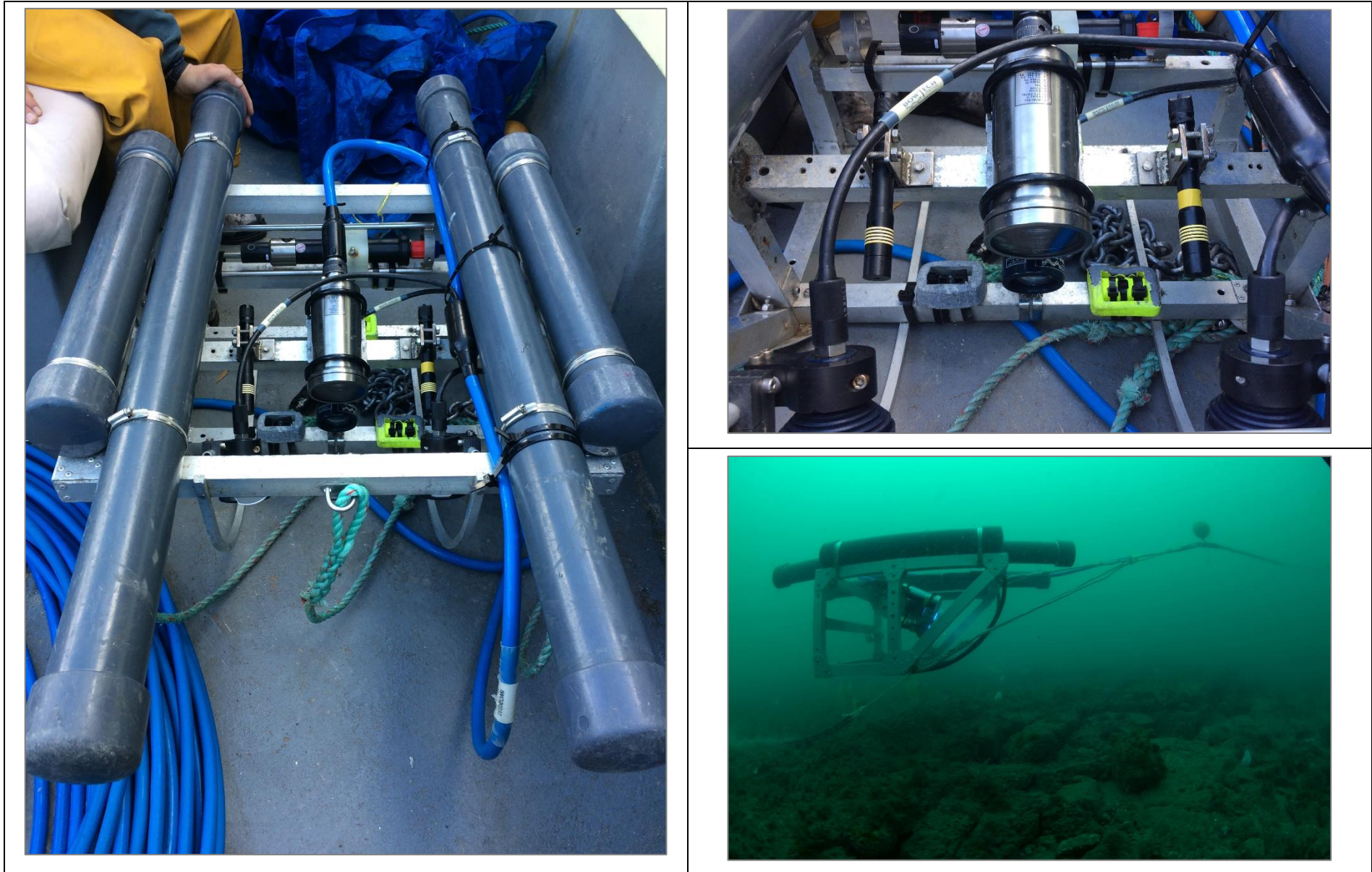
Figure 4. Left: TUV showing buoyancy tubes. Top right: Camera, lights and lasers on TUV. Bottom right: TUV deployment underwater (photo: University of Plymouth).
