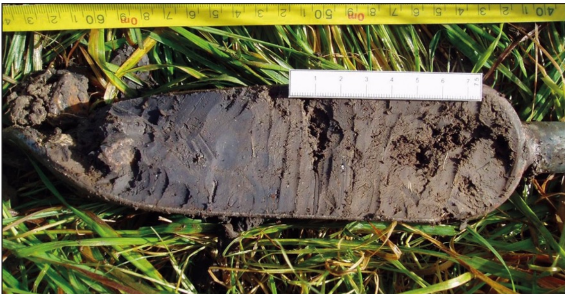
Figure 21: Ufton Bridge: black organic silty clay in hand auger chamber (photo M. Bell)
