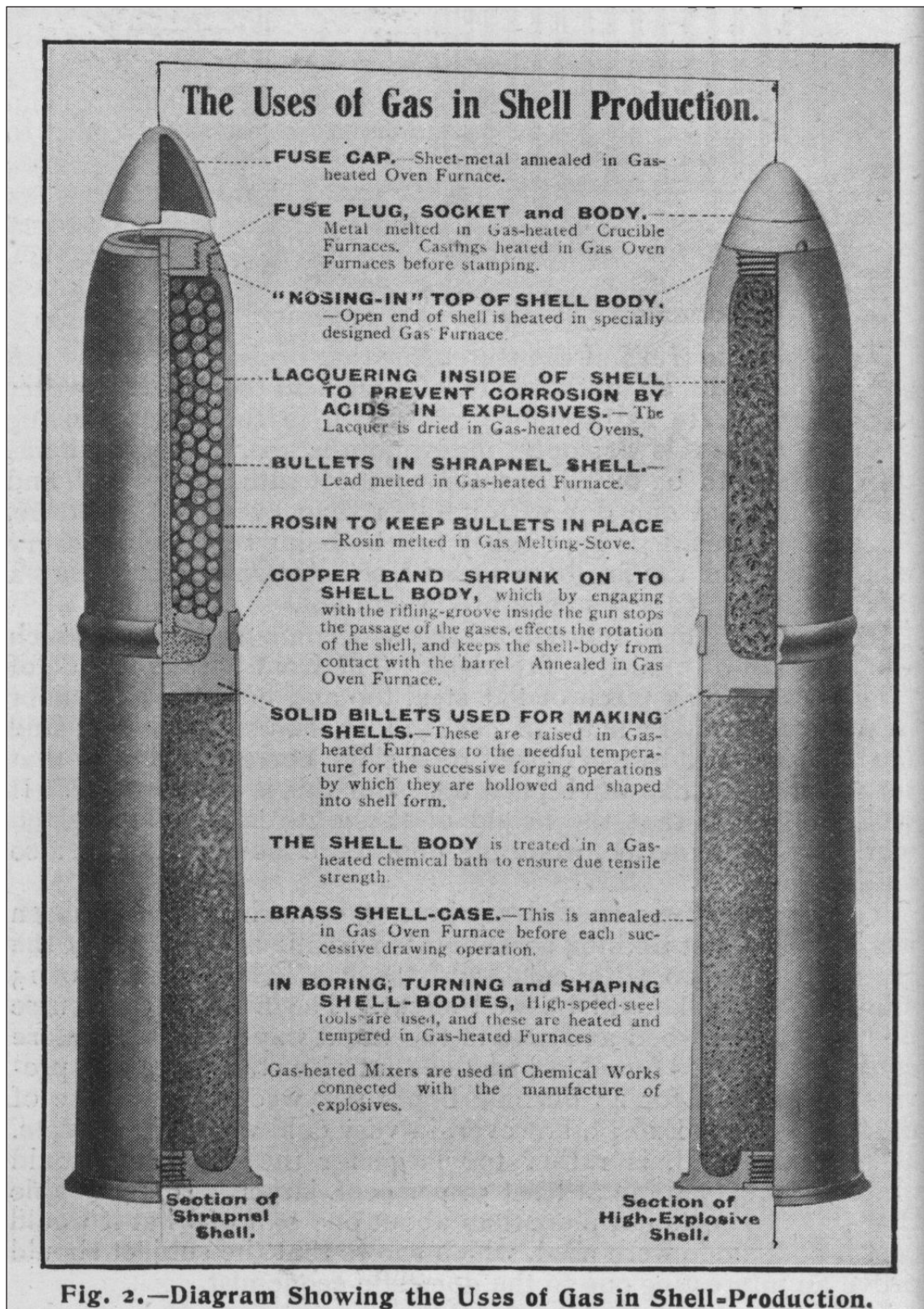
Figure 2.59 Showing the importance of the gas industry to the manufacture of shells during World War 2. Source National Grid Gas Archive.
