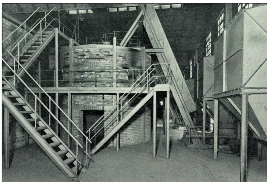
Figure 3.198 The Spent Oxide burners at the Kachkaroff plant of the East Greenwich gasworks, circa 1950. Image courtesy of National Grid Gas Archive.
