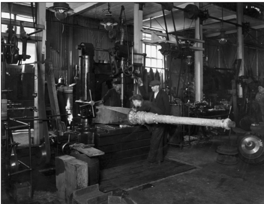
Figure 3.202 A gas lamp being repaired in a gasworks workshop. Image courtesy of National Grid Gas Archive.
