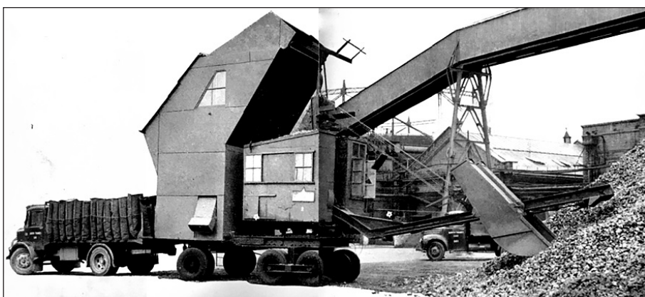
Figure 3.91 A mobile Harmer coke screening and bagging plant at Southend Gasworks circa 1950s. Image courtesy of National Grid Gas Archive.
