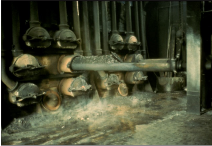
Figure 3.27 Loading a retort with a mechanical charger. Image courtesy of National Grid Gas Archive.
