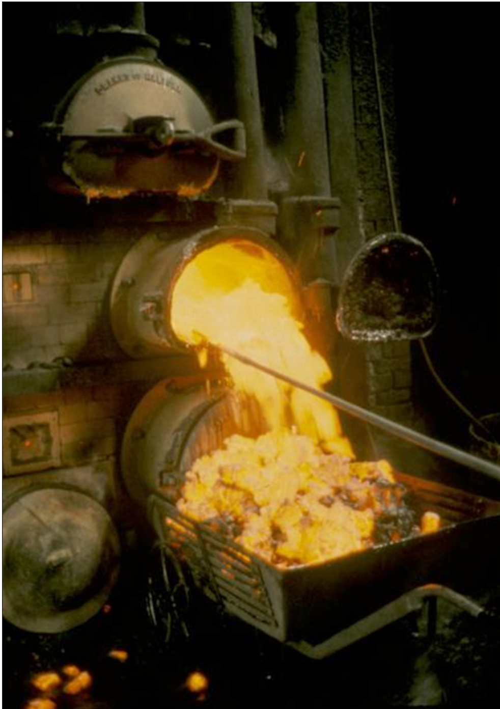
Figure 3.24 Manually emptying hot coke from a stop-ended horizontal retort. Image courtesy of National Grid Gas Archive.
