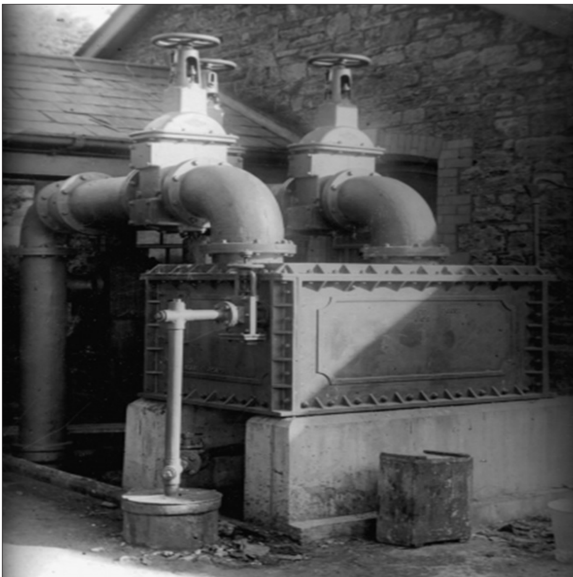
Figure 3.66 A Livesey washer. Image courtesy of National Grid Gas Archive.
