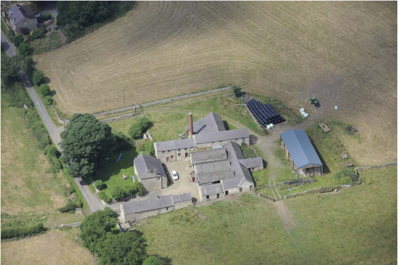
Steam-powered farmstead of c 1860-70 (note the chimney at the junction of the barn and mixing house range) at Shildonhill. Photo © Historic England 28561/010
