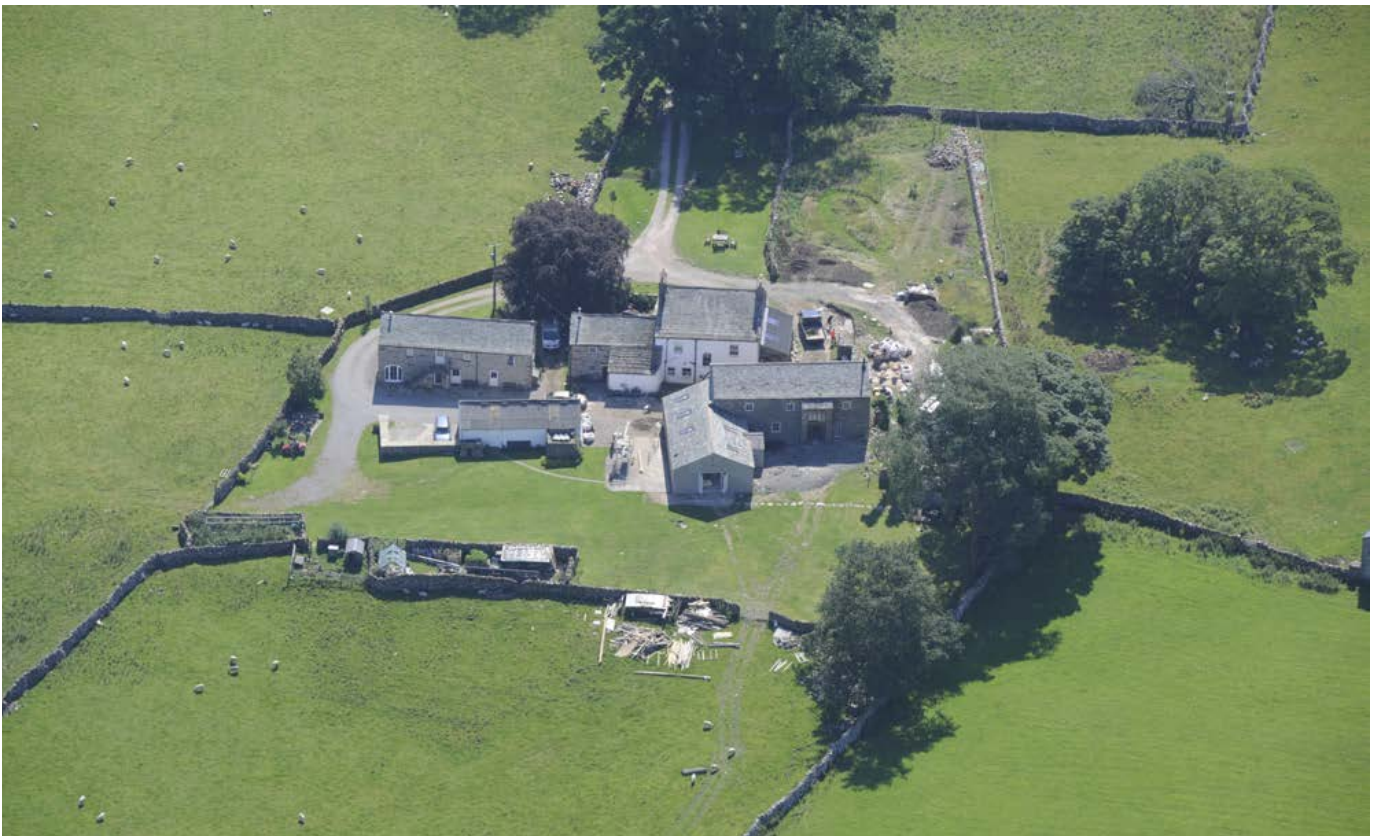
One of the farmsteads shown on the front cover. This is a clustered group of late 18th- and 19th-century buildings dominated by two large combination barns for housing cattle, storing hay and processing corn. Note the sheep pens and the detached field barn. The house was rebuilt in the early 19th century, around an earlier core, and faces away from the farmyard into its own garden and the public approach. Photo © Historic England 28572/056
