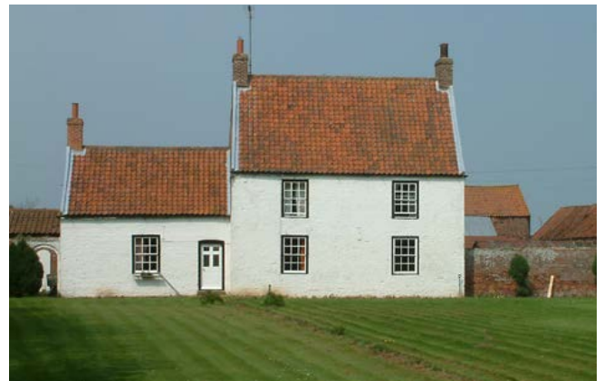
Isolated 18th-century steading with regular yard arrangement of single and two-storey buildings set behind the farmhouse. Note the steeply-pitched pantiled roof, characteristic of the area. Pantiles with their distinctive wavy profile and orange/red colour are the dominant roof cover, virtually replacing thatch by the 19th century. Photo © Jen Deadman
