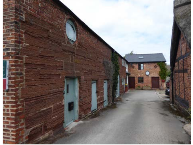
This group to the west of Tarvin illustrates the range of materials available in this area – timber-frame, as commonly used into the early 18th century for farm buildings, coursed and dressed sandstone and brick which was used for high-status houses from the 17th century. Photo © Jeremy Lake
