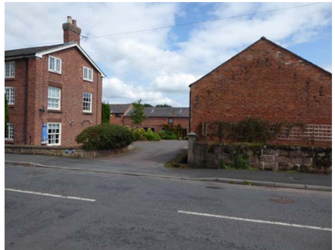
This group to the west of Tarvin illustrates the range of materials available in this area – timber-frame, as commonly used into the early 18th century for farm buildings, coursed and dressed sandstone and brick which was used for high-status houses from the 17th century. Photo © Jeremy Lake
