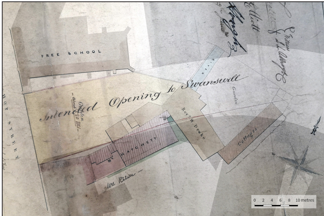
Figure 36: 1846 'Plan of Intended Street' overlaid on modern OS mapping (grey). Note that the rear elevations of number 3-9 (odd) Hales Street correspond to their existing alignment, with the fronts of the properties apparently being realigned and/or refronted to accomodate the road.
