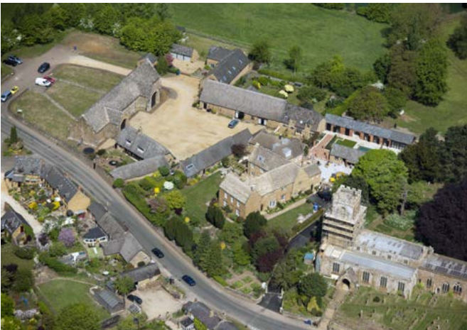
The russet-coloured stone used for the barn at Swalcliffe in Oxfordshire, like the other traditional buildings in the village, is typical of the area around Banbury and extending northwards into the Northamptonshire Uplands. The barn of c.1400 was always the principal building within this loose courtyard arrangement of buildings, which were built to serve the estates of New College in Oxford. Photo © Historic England NMR 26946 011
