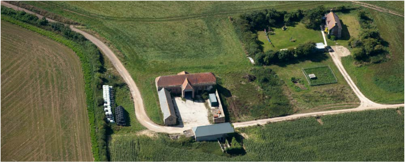
A former regular U-plan farmstead with a five-bay threshing barn, a cattle shelter shed to one side, now missing its roof, and stabling opposite built as part of the enclosure of common land at Vines Down in the 19th century. Photo © Historic England 27842/004
