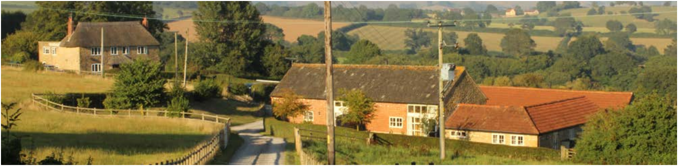
A mid- to late 19th-century, regular courtyard group with an L-plan range and a detached building to the third side of the yard. The large glazed opening is a modern insertion giving what was a two-storey cow house a barn-like feature. Photo © Bob Edwards
