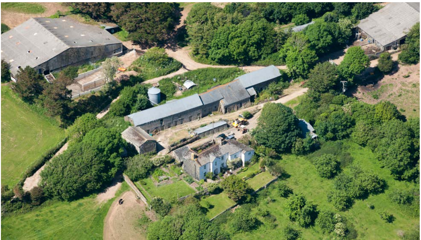
This farmstead at Osborne Newton is dispersed along a driftway, this being a type of plan found in areas where farms developed alongside routeways for moving stock to moorland grazing areas. The high-status, 17th-century house looks out over remnant orchards. The long range includes a combination barn, shippon (cow house) and stables. Photo © Historic England 29061/040
