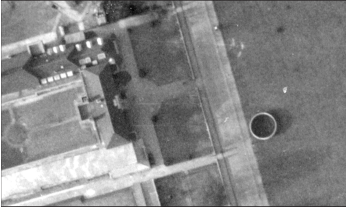
Figure 89 – Circular Emergency Water Supply (EWS) photographed in 1946 opposite what is now Chislehurst School for Girls. Detail of RAF/106G/LA/1339 RV 6301 29-MAR-1946. Historic England Archive (RAF Photography)
