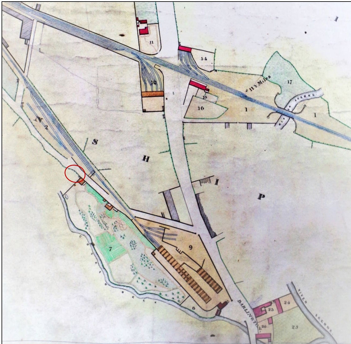
Figure 4: Thomas Dixon plan, surveyed 1839. The layout of the original depot at the terminus of the Darlington branch line with two parallel lines of ‘cellars’ which were filled from waggons with bottom-opening doors. Horse-drawn carts would approach from either side for loading coal from the cells and then re-join the Great North Road (now North Road). The building at the entrance to the depot was the lodge and weigh house. Position of later Lime Depot circled (TNA RAIL 1037 456 and 1037/482, reproduced with permission)
