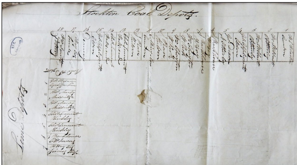
Figure 8: Plan of Stockton Coal and Lime Depot from February 1830 showing a larger number of coal cells along the top and the lime cells to the left, storing lime from Middridge and Thickley where quarries had been opened and kilns burned since 1826. 16 (TNA RAIL 667/1359, reproduced with permission)
